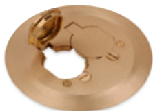
P60-CACP One-piece solid-brass duplex plate with screw-lock lids. 5 7/8" O.D. Mounting holes on a 3 3/4" dia.
