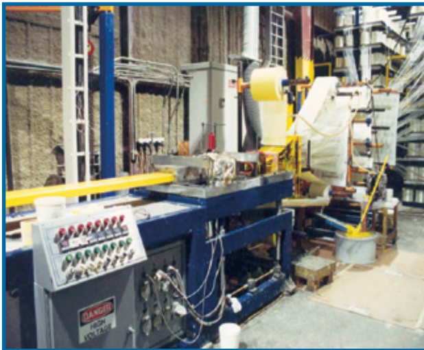
A surface veil is applied during the pultrusion process to ensure a resin-rich surface for superior corrosion resistance as well as an ultraviolet exposure barrier.
