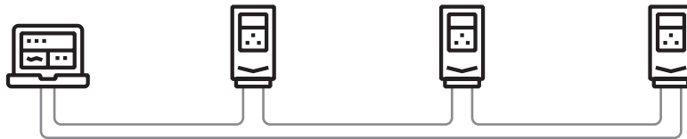
DDCS ring network. PC uses USB or PCMCIA adapter.
