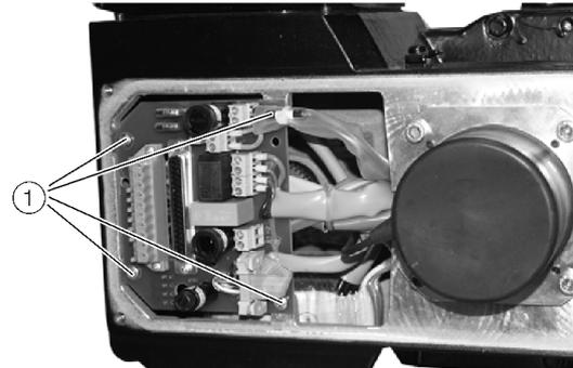
Figure 32: Removal of connection pcb at PME120-AI
