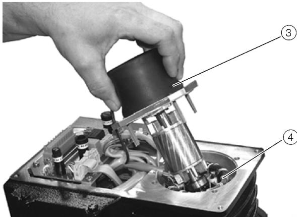
Figure 13: Brake body with rotor
