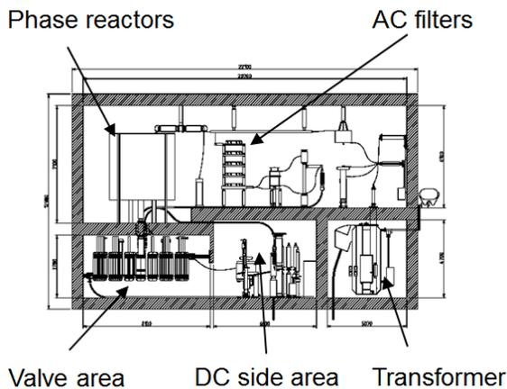
Figure 3. Layout of offshore converter
