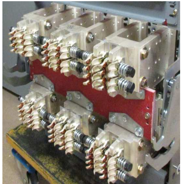
Figure 7A. AKD-10—Primary Contacts or “Fingers” (Apply Grease)
