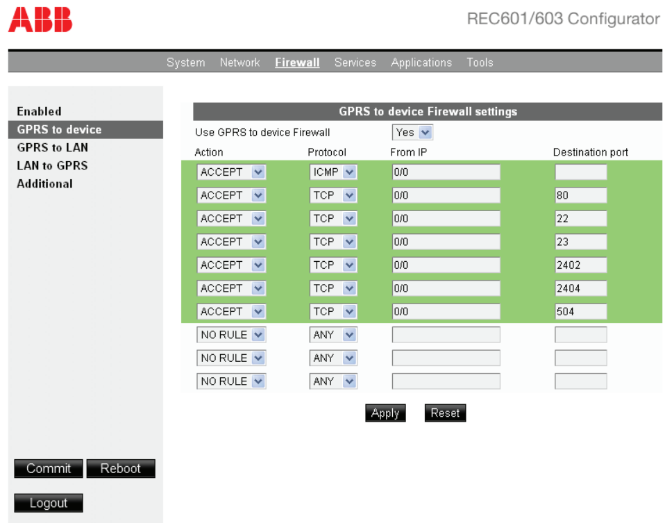
Figure 29: GPRS to device firewall settings
