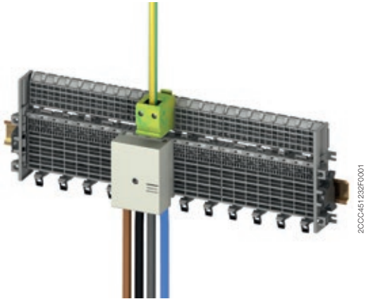
Power supply in centre, maximum 160 A. A maximum of 100 A is permitted on either side. A total of 160 A must not be exceeded.
