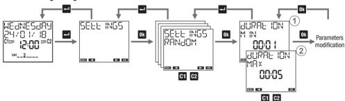
The "random switching  $\odot$ " function (activated with the combination described on page 6) allows the channel on which it's active to automatically switch and at random time intervals.
