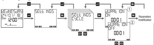
The "cycle switching" function (activated with the combination described on page 6) is a succession of on and off switching. The cycle programme always starts from the on status. In this menu it's possible to define the duration of on and off.
