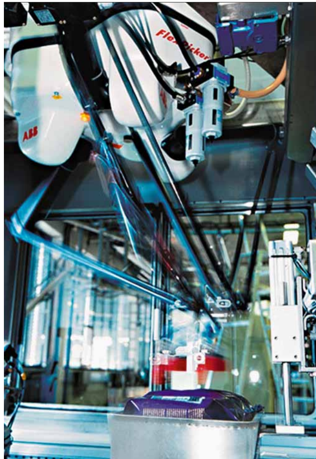
5 IRB 340 case-packing coffee at Löffbergs Lila, Sweden
