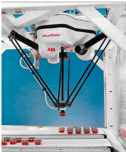
2 IRB 340, a parallel arm design
