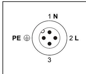
The illustration shows the pin side of plug **1** on the analyzer module.
