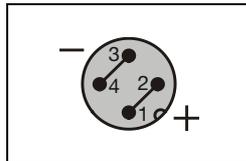
The illustration shows the pin side of the analyzer module 24 V DC plug and thus the solder side of the matching female jack.
