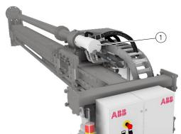
2. Remove cover (1) to access the center pipe inspection port(2) located at the end of the center pipe.
