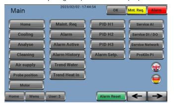
The illustration above shows the Menu page with error indication at the top right corner (in this example there are no active alarms, therefore the system is in normal state.
