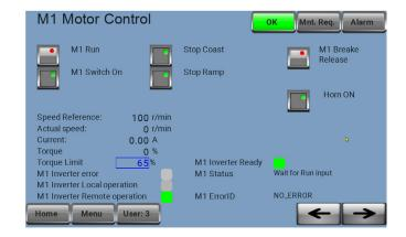
The above menu gives access to motor performance data and overload conditions. Various override functions are available for users with the right access level. Motor status and frequency drive error messages can be read.
