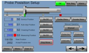
**WARNING!** The probe moves out of the kiln. Do not stand in the area of travel of the probe or probe buggy until the probe has reached its end position.
