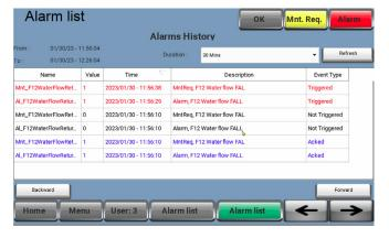
Red: Alarm active, not acknowledged Black: Alarm active, acknowledged Purple: Alarm not active, acknowledged
