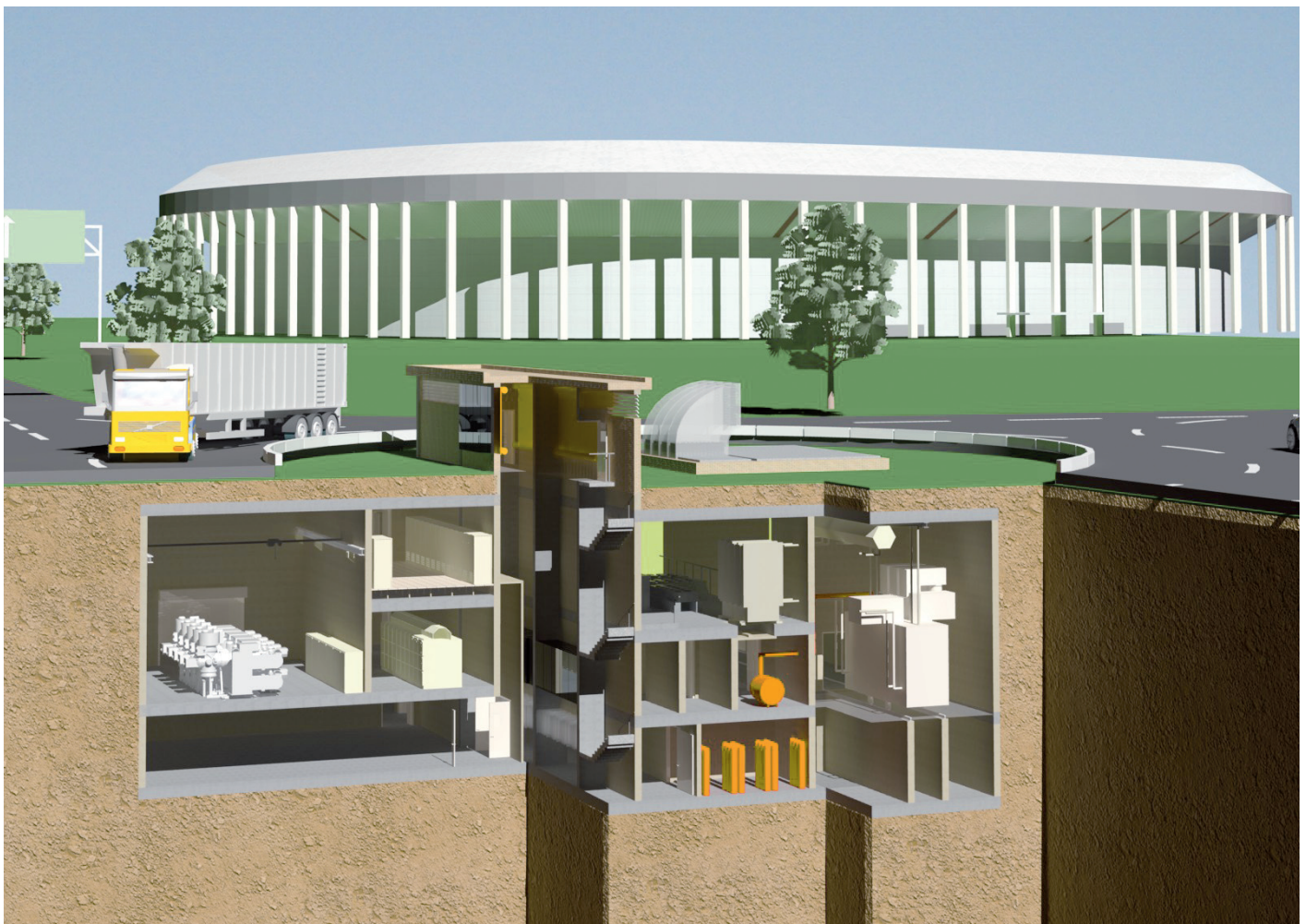
Locating transformer substations underground (here underneath a roundabout) offers more scope for urban planners.
