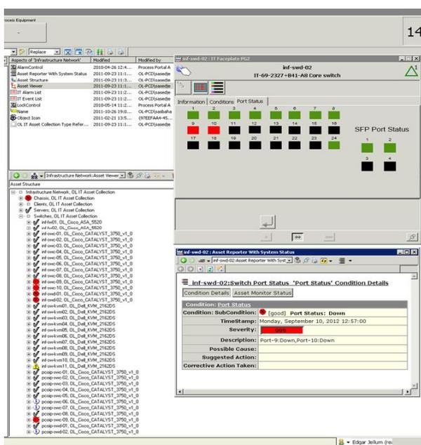
Figure 14: IT equipment and network asset monitoring
