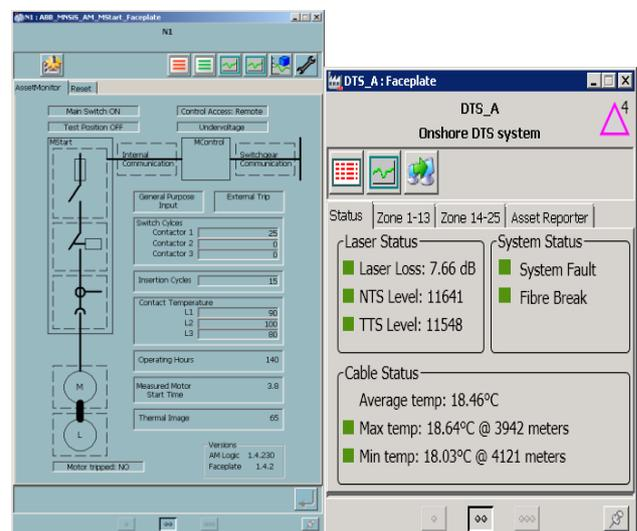
Figure 10: Contactor and DTS asset monitoring faceplates
