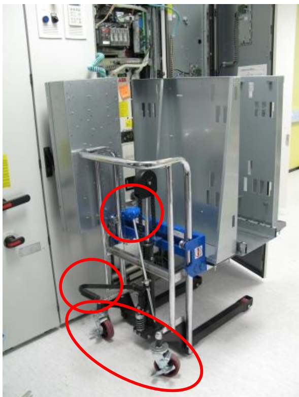
Picture 1: Locations of lowering knob (uppermost), lifting pedal (middle) and brake pedals (lowest)
