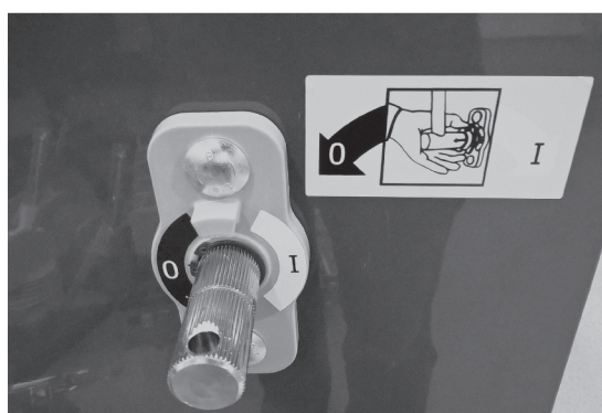
22 The shaft should loosely rotate loosely after taking out the arrestor ring
