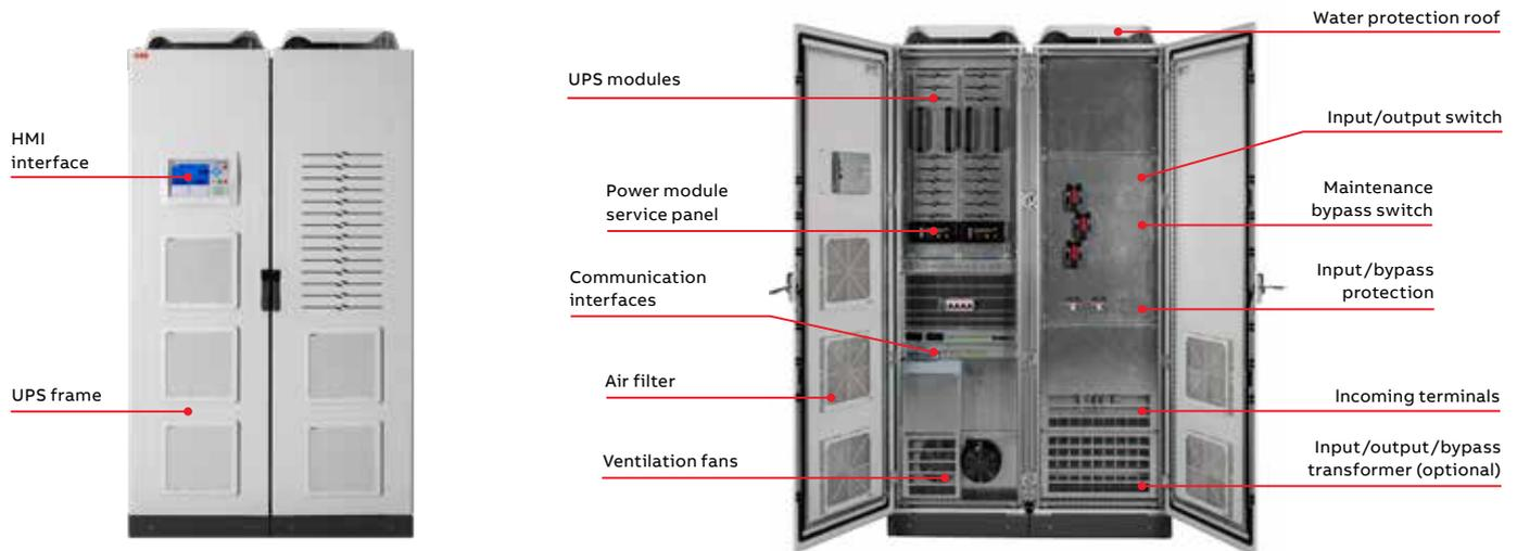
PowerLine DPA (3ph and 1ph) is an online double conversion UPS and makes the advantages of ABB's unique modular UPS architecture available for locations that are usually rough on electronic equipment. PowerLine DPA is based on ABB's Decentralized Parallel Architecture (DPA) that ensures the very best UPS design in terms of availability, serviceability, safety and ease of use.
