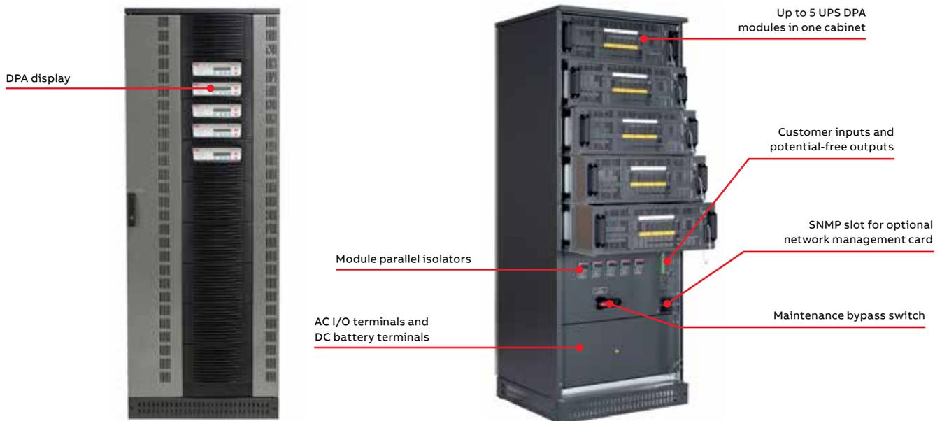
The Conceptpower DPA is a true double conversion modular UPS designed for medium-sized critical applications. The Conceptpower DPA's modular architecture provides very flexible power configuration based on 30 / 40 / 50 kVA modules that can be added as power requirements grow –
