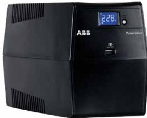
Intended for users with lower power requirements, the line-interactive PowerValue 11LI Up delivers from 600 up to 2,000 VA electrical power, making it the ideal UPS for modest IT applications. As well as intervening within 2 to 6 ms to power your application when mains power is lost, the PowerValue 11LI Up also filters out input power disturbances such as surges, line noise or brownouts. If the input power factor starts to play up, the PowerValue 11LI Up will automatically correct it.
