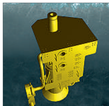
NuDeep tree. The traditional choke location on the tree has been moved to the manifold or integrated in the jumper systems.
