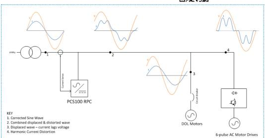
The diagram shows loads with both reactive and harmonic currents. Without a PCS100 RPC installed this current is sourced from the utility. With the PCS100 RPC installed the waveform is corrected at point 1 (utility).
