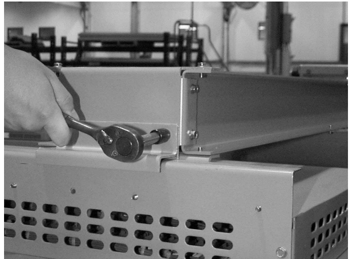
Fig. 4-23. Replacing the runner guide after completion of hoist installation
