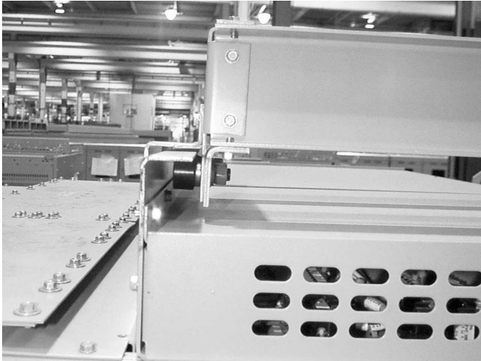
Fig. 4-21. Location of hoist rear rollers
