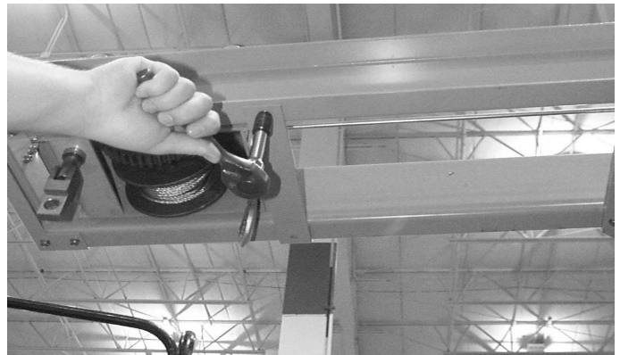
Fig. 4-24. Removing the bracket locking the hoist dolly
