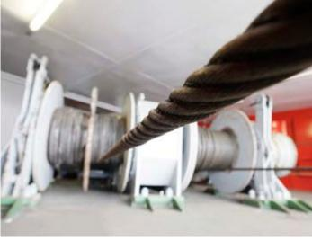
The existing motor, motor cable, mechanical disc brake and operator control stand were reused.
