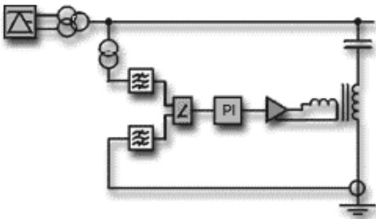
Fig. 2 Principle of continuous tuning
