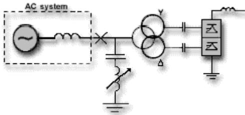
Fig. 5 Commutation capacitors are connected between the valve bridge and the converter transformers
