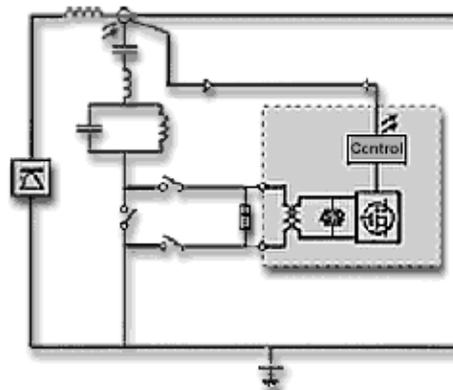
Fig. 4 Circuit diagram of active DC filter
