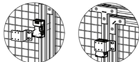
7. Make sure all screws are tightened and hammer nuts turned out correctly in the aluminium profile. Check the function by opening and closing the door a couple of times. Adjust the Z-bracket with actuator if needed.
