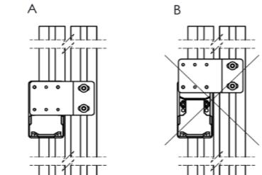
4. The standard key can be mounted in several different ways depending on how the switch is mounted on the fence and whether the door is right-or left handed. Please find mounting examples below.
