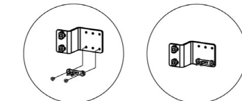
6. Mount the Z-bracket with actuator on the door leaf. Adjust the Z-bracket until the actuator slides perfectly into the actuator opening of the switch.
