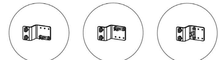
5. Mount the standard key onto the Z-bracket using the M5x8 screws (2x).
