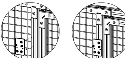
3. To reduce the risk of manipulation, mount the standard key (actuator) onto the Z-bracket according to example A below, in order to cover the mounting screws of the switch with the Z-bracket.
