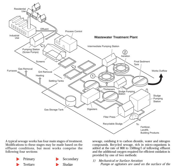
Sewage works are frequently divided into types, normally based on the method of the secondary treatment, with similar installations for the remainder of the treatment.
