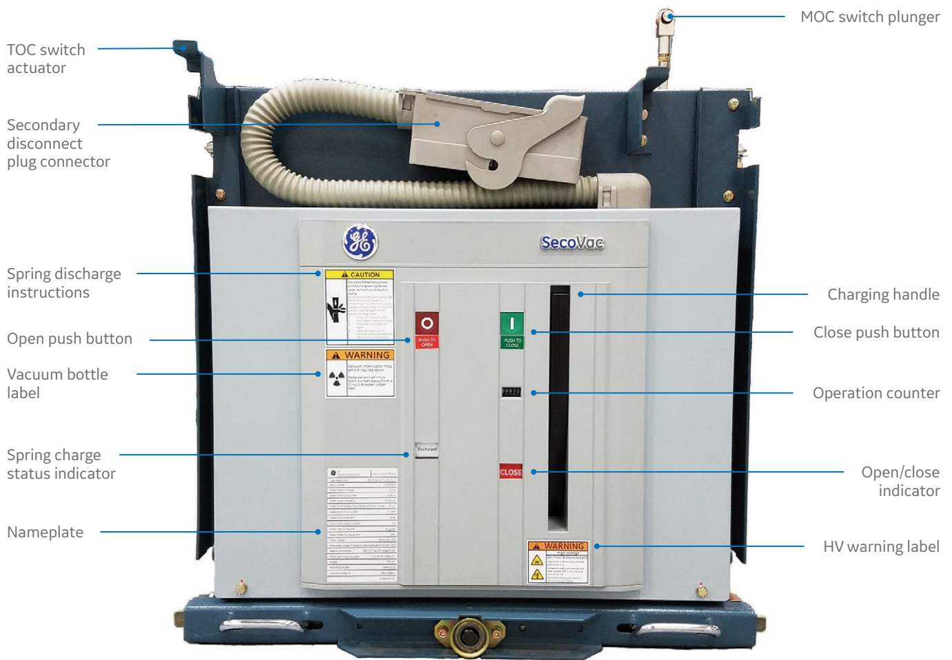
Figure 3-15: SecoVac Vacuum Circuit Breaker
