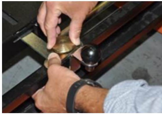
Figure 5-16. Press Down on the Interlock Pin and Rotate Clockwise to Lock the Latch Handle
