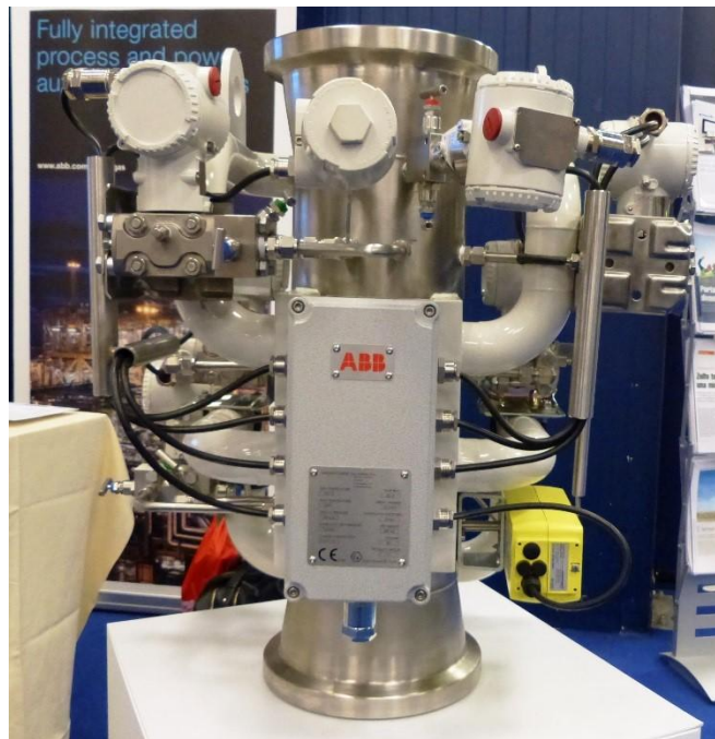
Figure 2 – The new VIS multiphase flowmeter
