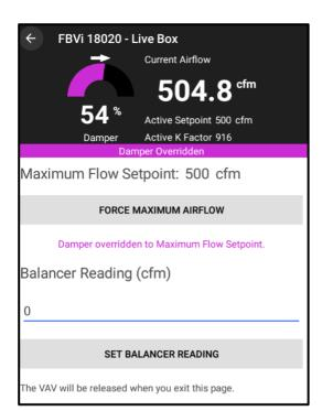
The color of the damper position will change to purple, indicating the unit is not in auto mode and is being overridden.
