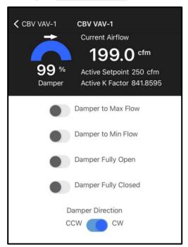
Switch to force Damper to Max Flow Setpoint.
