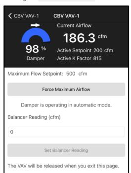
Step 1 – Verify your minimum flow setpoint. This can be set by returning to the main screen and selecting FLOW SETPOINTS
