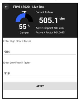
Enter both the high and low K Factors for the VAV. For maximum flow, this is available from a chart mounted on the side of an installed VAV, or from documentation from the unit manufacturer.
