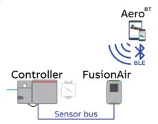
Regardless of the method of finding controllers (Wi-Fi or BLE), the same controller will be found. You may start with BLE to work with a controller. Later as Wi-Fi becomes available, you may search and find the same controller. Later still, if you need to access the controller again and would like to use BLE, you may switch to BLE and find the same controller. (The serial number of the controller is used as the key).
