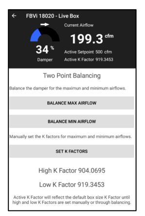
If both the min and max airflow has been balanced, the Active Setpoint will show the calculated K Factor, which will actively reset between the Low K Factor and the High K Factor.
