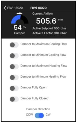
Switch to force Damper to Max Cooling Flow Setpoint.
