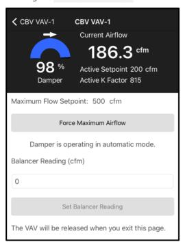
Step 1 – Verify your maximum flow setpoint. This can be set by returning to the main screen and selecting FLOW SETPOINTS
