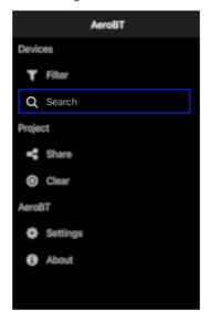
When configured for Wi-Fi, the Search option allows you to search the network for Controllers. When controllers are found, they will be added to the All Devices page.
