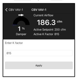
Enter the K Factor number for the VAV. This is available from a chart mounted on the side of an installed VAV, or from documentation from the unit manufacturer.
