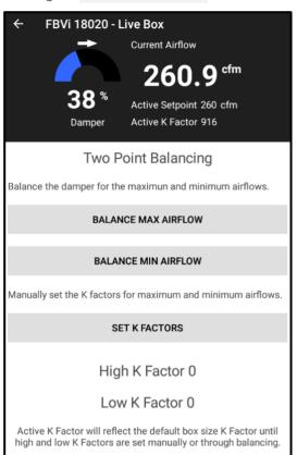
Step 1 – Verify your maximum flow setpoints and minimum flow setpoints. This can be set by returning to the Main Screen and selecting FLOW SETPOINTS
