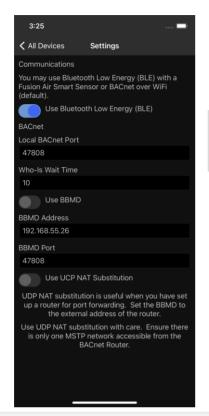
Use Bluetooth Low Energy (BLE) – To use BLE, toggle this option on. Wi-Fi will not be used to search for and communicate with controllers. Instead, **FusionAir** Smart Sensors will be used to communication with the controller the sensor is connected to.
