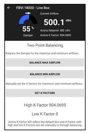
If the max airflow has been balanced, the Active Setpoint will show the calculated maximum K Factor. It can also be read from the Two Point Balance screen.
