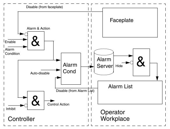
Figure 111. Inhibit and disable functions in alarm handling for AC 800M (for a list of objects with inhibit functionality, see Inhibit Parameters on page 256). Event handling works in a similar way.
