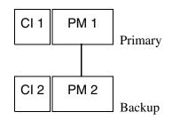
*Figure 173. A schematic illustration of a redundant controller configuration before start of Online Upgrade.*
