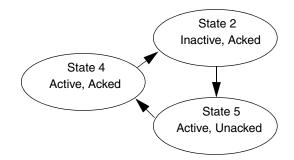
Figure 128. State diagram for enabled alarm conditions with AckRule 1, part 1.
