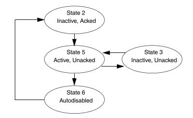
Figure 130. State diagram for enabled alarm conditions with AckRule 1, part 3.
