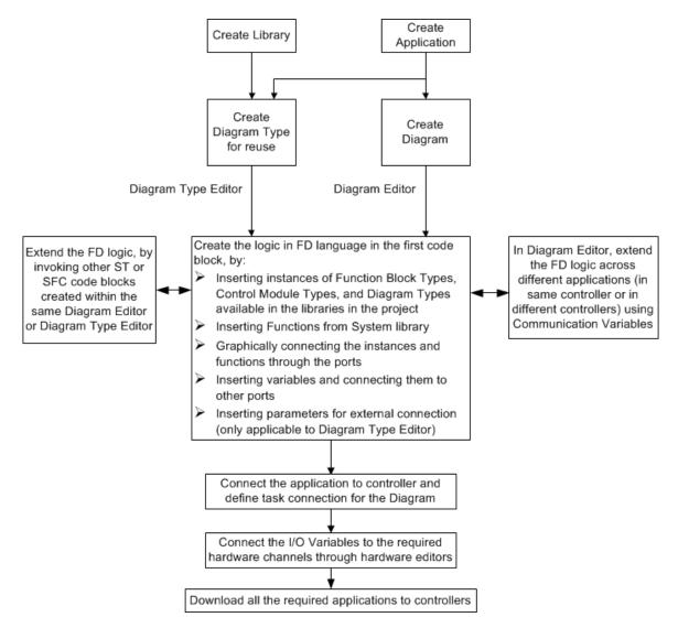
Figure 16. Workflow for using Diagrams and Diagram Types
