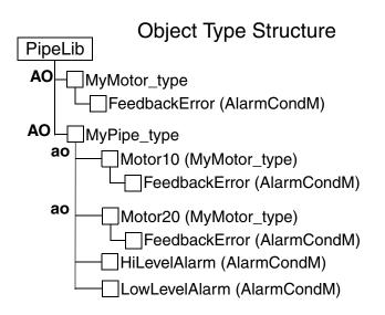
*Figure 123. PipeLib. AO=Alarm Owner (setting in type), ao=alarm owner (setting is inherited from type).*
