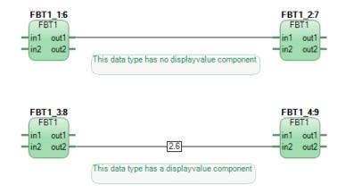
Figure 150. Graphical connections of structured data type
