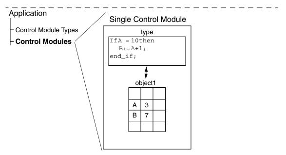
*Figure 24. A single control module. This module is not reusable, hence intended to be used only once for grouping instances into a single unit.*
