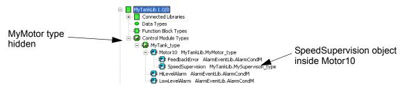
*Figure 59. The Hidden attribute on MyMotor type would still allow showing objects (children) of the MySupervision type in any new motor object.*
