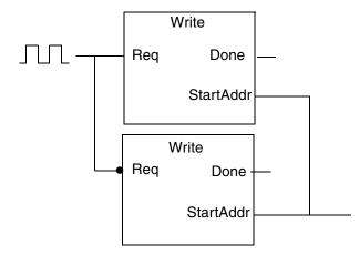
Figure 143. Resetting the Req parameter using two function blocks.
