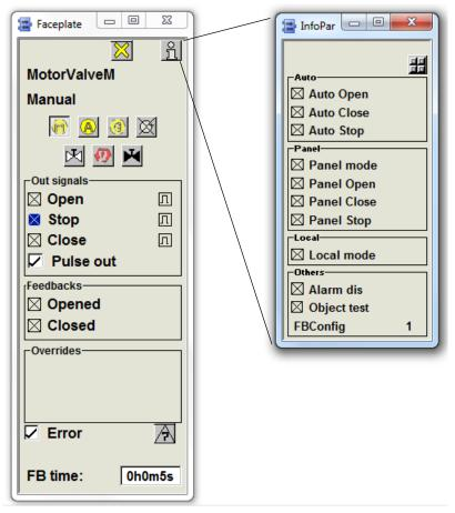
Figure 158. The left window is an interaction window activated from an application window interaction object. The right window (supervision only) appears after clicking the info interaction window button.
