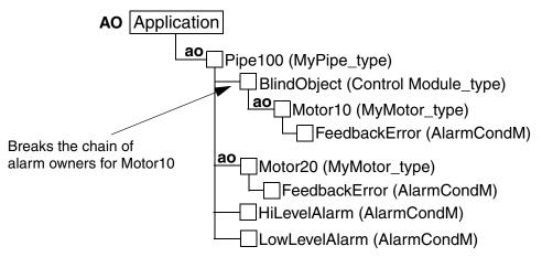
Figure 125. Inserting a "blind object" to break the alarm owner chain.
