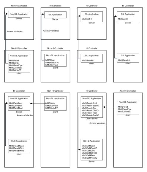
Figure 146. How to choose MMSCommLib function blocks/control modules.
