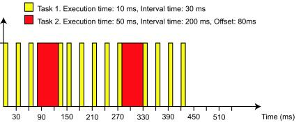
Figure 65. Execution of two tasks with the same priority.
