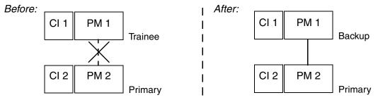
Figure 176. The redundancy has been re-established.
