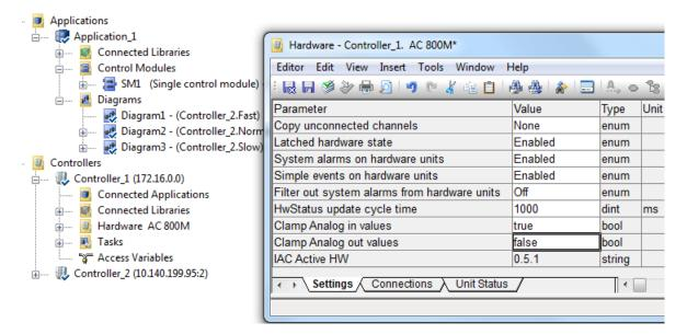
Figure 90. Enabling over and under range for output objects
