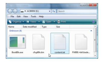
Figure 96. Firmware image files on SD card
