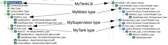
*Figure 56. A Library structure before any protection attributes have been set. (Left) Project Explorer tree. (Right) Object Type Structure in Plant Explorer.*
