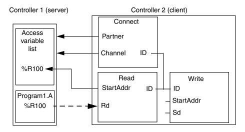
Figure 142. Variable read by controller 2, from controller 1.
