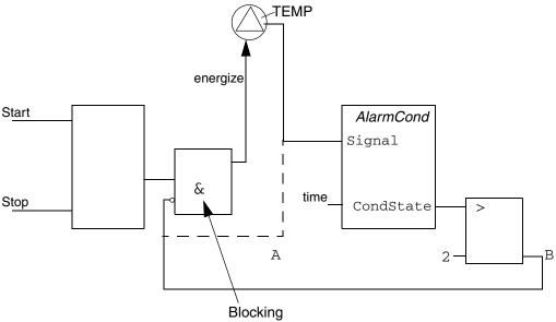
Figure 126. Manipulating the condition state using I/O.
