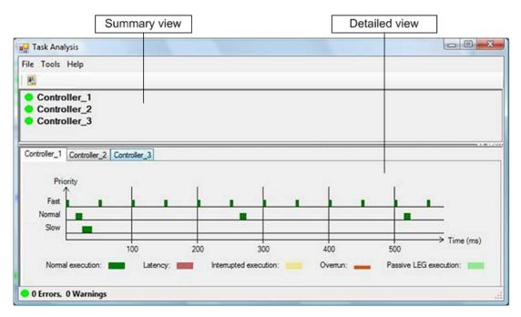
Figure 72. Task analysis tool opened from Tools > Task Analysis
