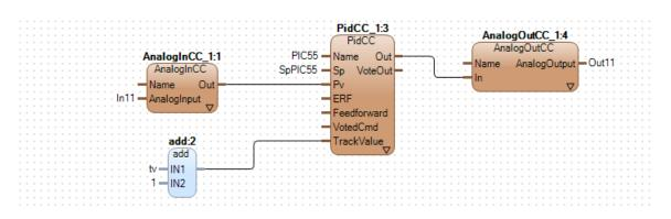
Figure 12. Example logic created in the graphical code pane of diagram type editor
