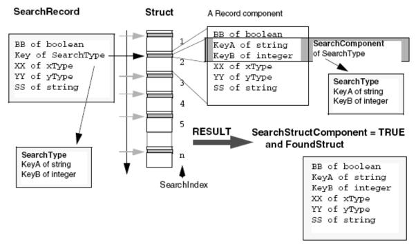
Figure 192. The working principal of the SearchStructComponent.
