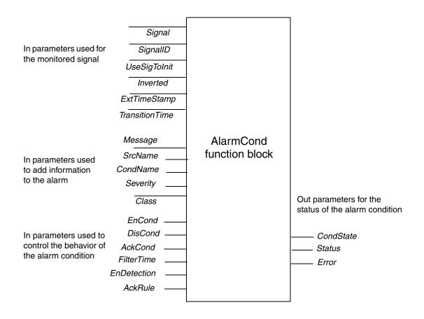
Figure 110. The function block AlarmCond.
