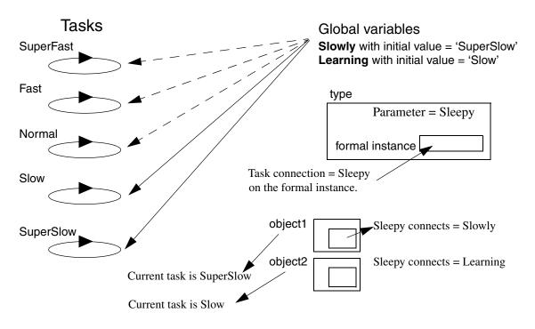
Figure 32. Each object can be connected to a different task via the parameter Sleepy declared in the type and task connected in the formal instance.
