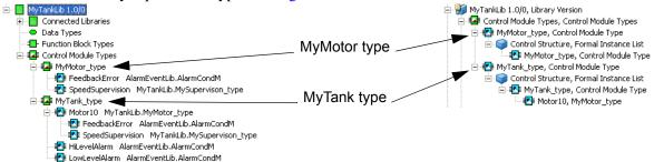
Figure 57. MySupervision\_type is not shown in Plant Explorer after setting the hidden attribute. (Left) Project Explorer with SpeedSupervision still visible. (Right) Object Type Structure where both MySupervision\_type and SpeedSupervision are hidden.
