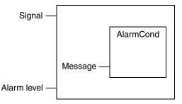
Figure 33. The function block AlarmCond located in the Alarm library.
