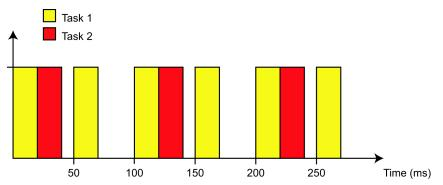
*Figure 67. No offset. The two tasks have the same priority, but different interval times (50 and 100 ms).*
