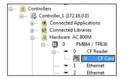
*Figure 91. The Controllers item expanded and the CF Card connected to the CF Reader item.*
