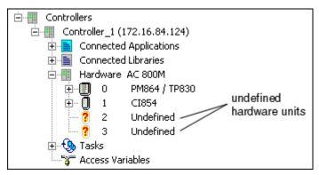
Figure 166. Undefined hardware units in Project Explorer.
