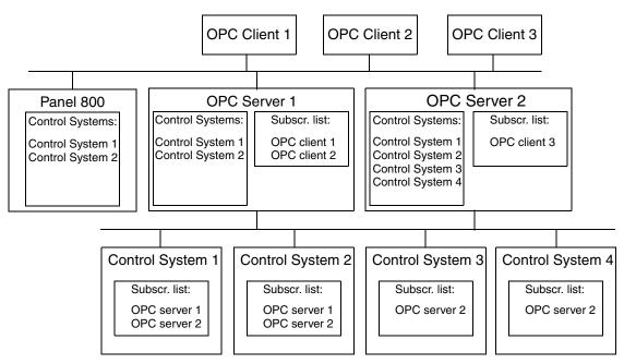
Figure 113. Example of a control network configuration.
