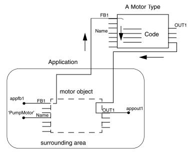
Figure 21. A control module instance connected to variables in an application. The application is the 'surrounding area' with the variables appfb1, Name (initial value 'PumpMotor') and appout1 connected to the instance.
