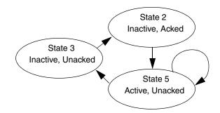
Figure 134. State diagram for enabled alarm conditions with AckRule 5, part 2.
