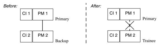
Figure 174. The redundancy is disabled and the backup is preparing for an upgrade. Thus the role switches from Backup to Trainee.
