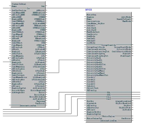
Figure 127. Example of how to implement inhibition of an alarm.
