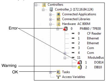
Figure 157. Status indications of hardware and tasks in Project Explorer.
