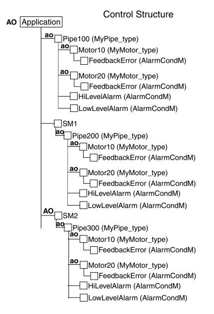
Figure 124. Three pipes with different alarm owner conditions.
