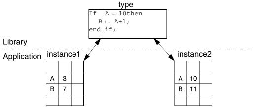
Figure 3. Relationship between a type and two instances.
