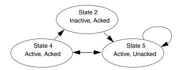
Figure 133. State diagram for enabled alarm conditions with AckRule 5, part 1.
