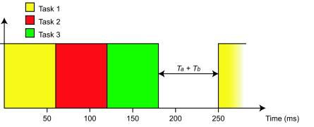
Figure 69. The result of having no offset for three tasks with long execution times. The gap  $(T_a+T_b)$  is the time available for the execution of other functions, for example communication.
