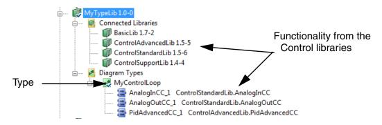
Figure 15. A Type (MyControlLoop) created in MyTypeLib library. This example shows a control loop created as a diagram type, while the components are ready-made instances from the standard libraries
