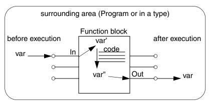
*Figure 22. In and Out parameters for a function block. This example illustrates how In and Out parameters copies the variable (var).*
