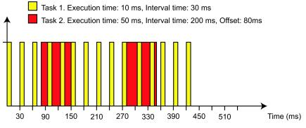
Figure 66. Execution of two tasks with different priorities.
