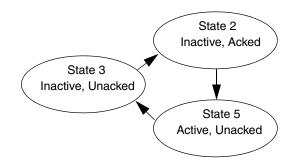
Figure 129. State diagram for enabled alarm conditions with AckRule 1, part 2.
