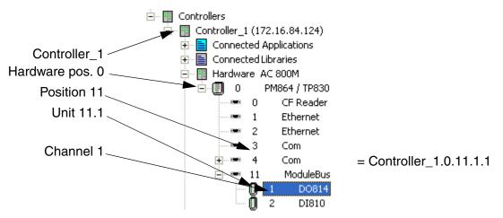
Figure 34. An example of how IO channel addresses are created in a control project.
