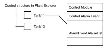
Figure 121. Aspect Object Tank11 in Plant Explorer, showing some aspects.
