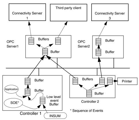
Figure 114. Example of buffer configuration. When a buffer is full, a system simple event is sent upward to the 800xA system and the third party client. In Controller 1, there is also a low level event buffer receiving events from an external device (in the example, an INSUM device).
