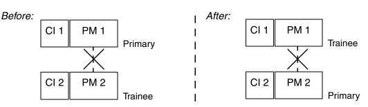
Figure 175. PM 1 and PM 2 are shifting roles. After this step the PM 2 will become the Primary and execute the running application.
