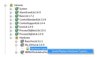
Figure 52. Inserting hardware types in library
