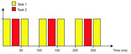
Figure 68. Offset is set on task 2. The two tasks have the same priority, but different interval times (50 and 100 ms) and are thus executed at the requested times.
