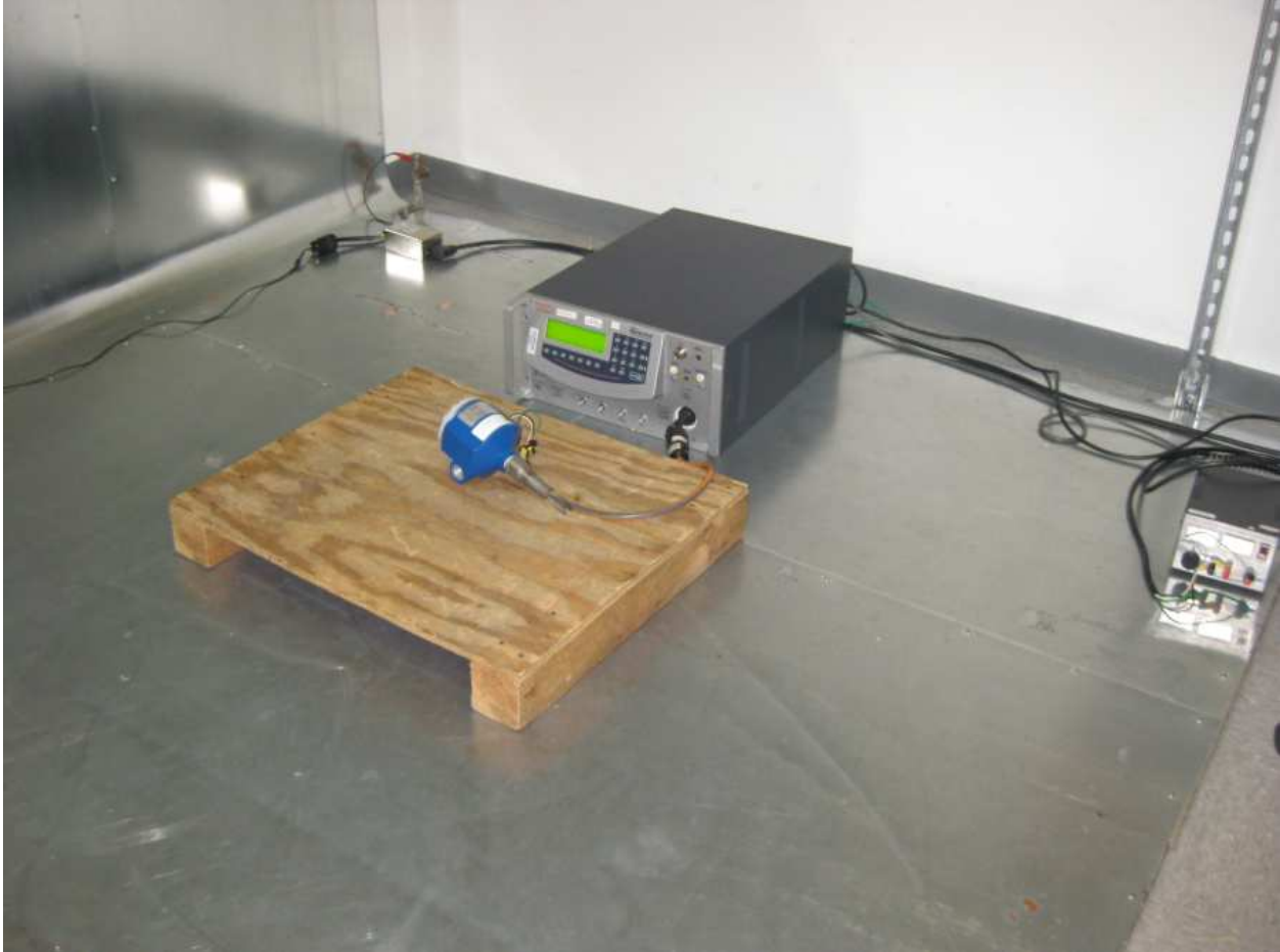
Figure 13-2 Electrical Fast Transients Test Setup
