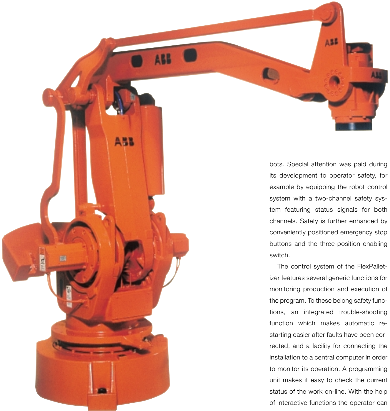
IRB 640 FlexPalletizer – the articulated system holds the rotary disc parallel to the horizontal plane, thereby replacing the otherwise usual but complex bend-back function and the wrist axis.
