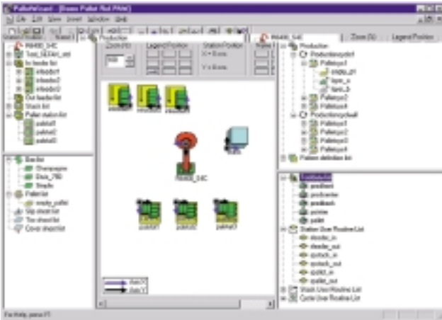
Five windows appear on the screen when PalletWizard is started. The middle window shows the workcell configuration, with icons representing three pallets and three infeed conveyors, plus a stack of empty pallets. The robot is also represented by an icon. 3
