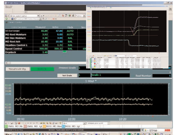
The operator's MD control window displays not only current, but also historical data, providing key information for necessary process decisions. Additional overlap displays allow simultaneous viewing of multiple process areas.
