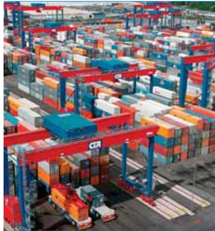
3 Automated handling of containers using automatic guided vehicles and automatic rail mounted gantry cranes
