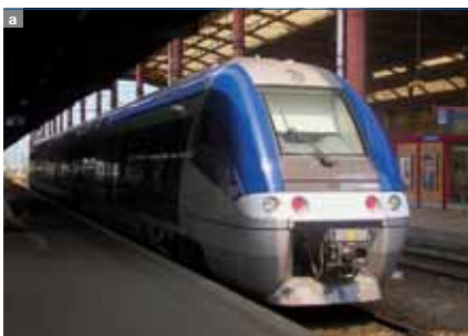
1 Modularity permits both diesel a and electric b variants of the AGC railcar for SNCF (French Railways). ABB is supplying the generators, transformers and traction motors.
