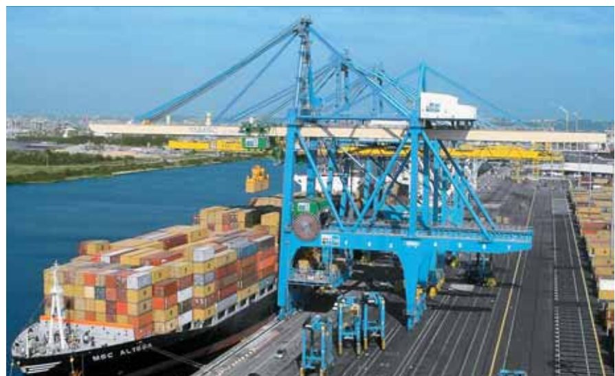
2 With modern ship-to-shore cranes a ship with 4000-5000 TEU (twenty feet equivalent) to unload/load can be handled in less than 24 hours
