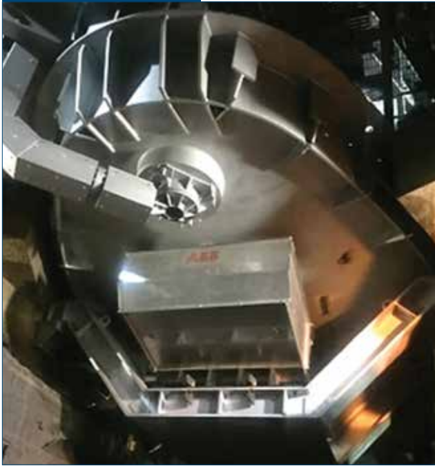
Arc furnace with ArcSave® stirrer mounted underneath the furnace bottom.
