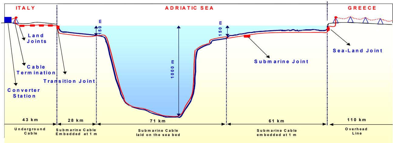
Fig.3 - The schematic bathymetric profile.
