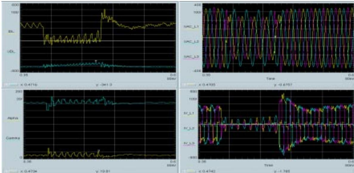
Fig.11 - Transient following AC remote fault at the Greek side.
