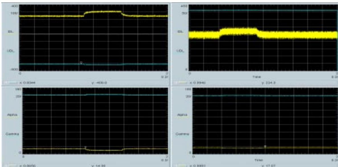
Fig.10 - Dynamic response to current steps of different amplitudes.
