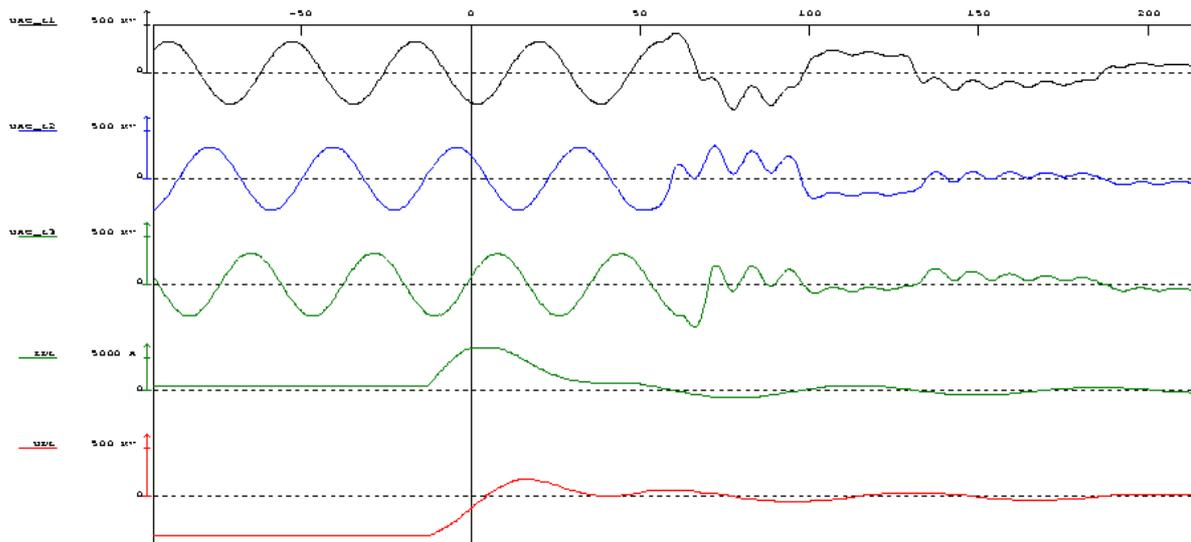
Fig.9 - Pole to ground fault applied on the valve side of reactor at the Galatina converter station.
