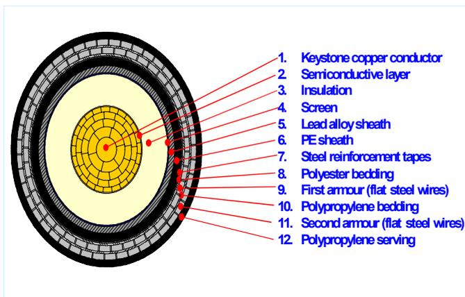
Fig. 4 – Submarine cable cross-sectional drawing.
