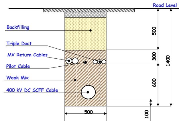
Fig. 5 – Land cable installation trench scheme.
