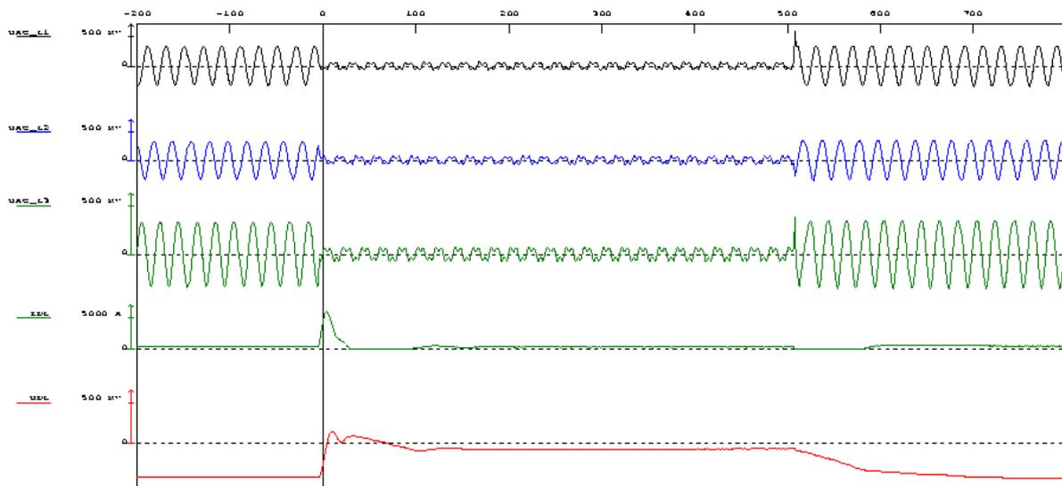
Fig.8 - 3-phase solid fault applied at the Italian network with Galatina operating as inverter.
