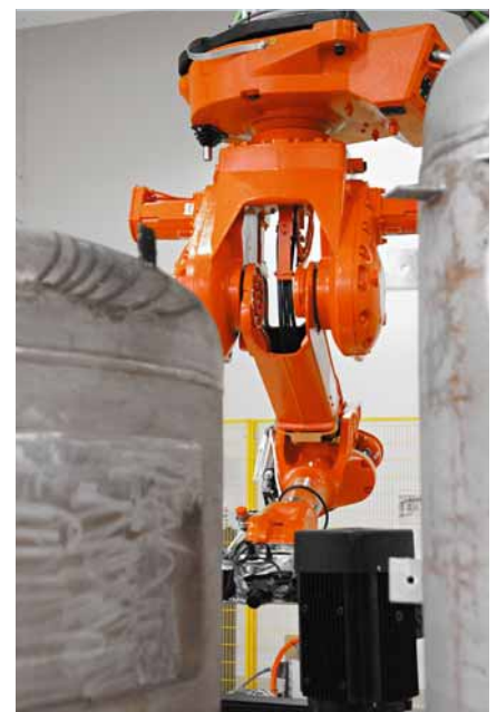
3 ABB robot at work performing routine inspection of process equipment
