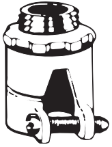
Straight squeeze-type connectors – malleable iron
