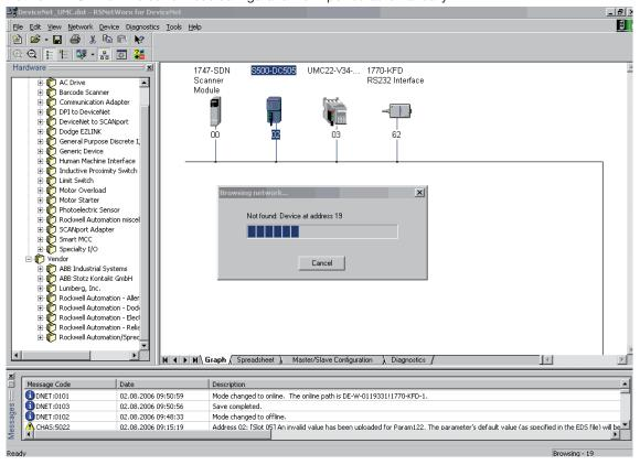
Then, you have to configure the devices and set the device parameters. For this purpose, open the device dialog by double clicking the corresponding device entry.
