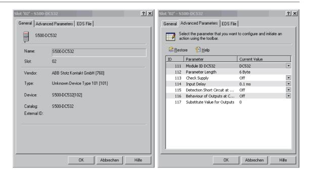
Confirm both dialogs with OK and click the Download button to download the changed parameters to the device.
