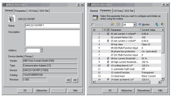
Open the "Parameters" tab and set the parameters as required for the application. After this, click the *Download* button to transfer all parameters or only individual parameters to the device.
