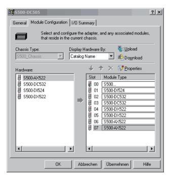
Open the properties dialog of the corresponding device by selecting *Properties* and edit the module parameters in the "Advanced Parameters" tab (refer to the following figures).
