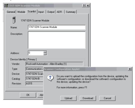
When opening the "Scanlist" tab for the first time, click the *Upload* button to load the current configuration stored in the master.
