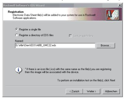
After the installation has been completed successfully, the registered new devices are available in RSNetworx.
