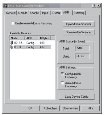
Highlight the entry of the device for which you want to activate the automatic parameter download and click the *Load Device Config* button.
