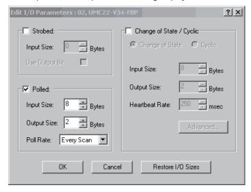
Now, you can use the "Input" and "Output" tabs of the DeviceNet master to specify the mapping of I/O data according to your PLC program.
