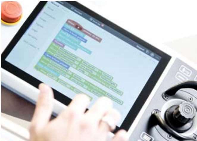
ABB's Wizard easy programming software is an ideal learning tool for those with little or no prior experience of robots.
