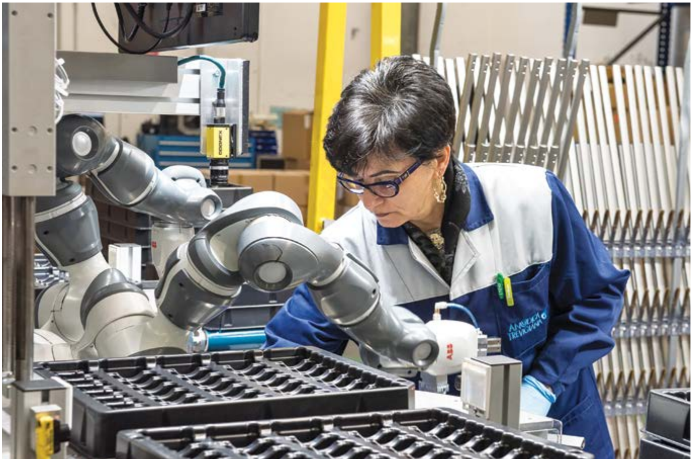
Italian manufacturer, Anodica, uses ABB's YuMi cobots to handle complex and repetitive production tasks, releasing workers for more interesting roles including supervising and programming the robots.
