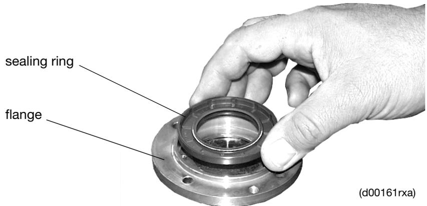
Fig. 6: Flange and sealing ring (exemplary picture)
