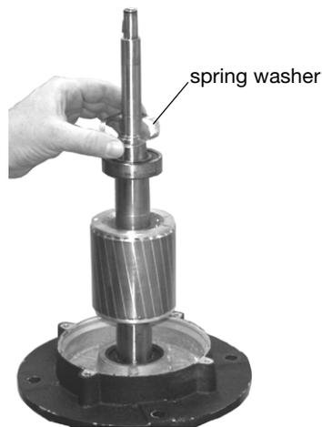
Fig. 22: pinion removal
