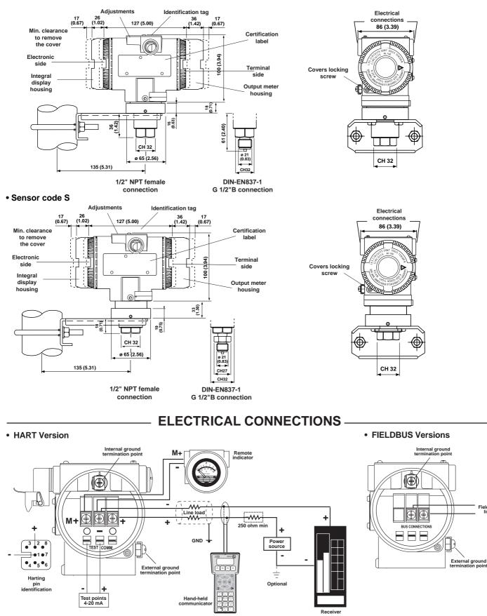
HART hand-held communicator may be connected at any wiring termination point in the loop, providing the minimum resistance is 250 ohm. If this is less than 250 ohm, additional resistance should be added to allow communications.
