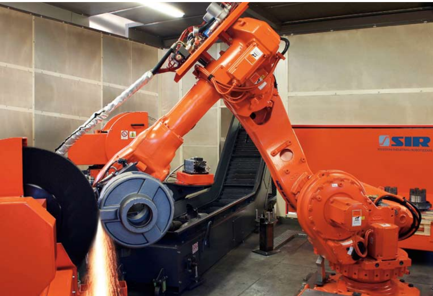
The milling and deburring units finish the piece to a precision of a few tenths of a millimeter with an IRB 6600 robot from ABB.
