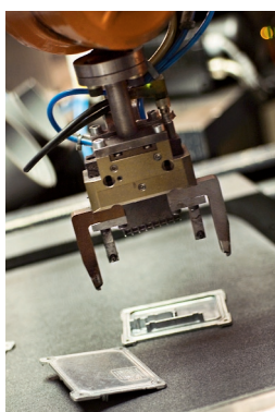
Aluminum components for automotive lighting systems are picked and placed by robots.
