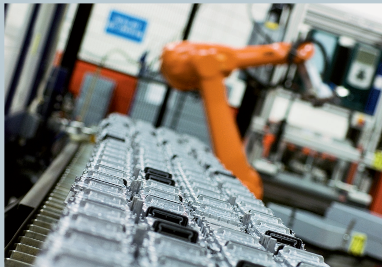
Some 30,000 PCB housing boxes for automotive lighting systems are produced each week at Stilexo.
