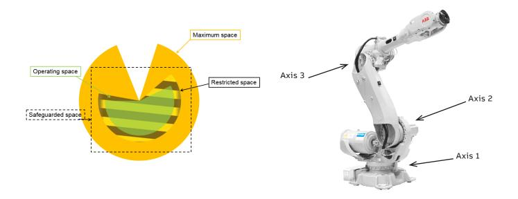
The standards EN ISO 10218-1 and -2 (harmonized standards to the Machinery Directive) give requirements on how to safely limit the space of the industrial robot.
