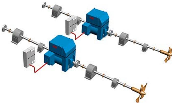
Figure 1: Overall principle of the shaft-installed electrical auxiliary propulsion system. The propulsion drive including the brake resistor (A) is fed from the auxiliary generator. The feeder may require a transformer to match the voltages. The drive feeds the auxiliary propulsion motor (B) when the main propulsion engine is disconnected from the shaft.
