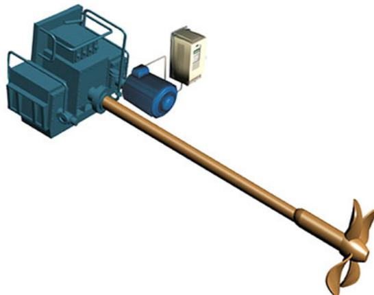
Figure 4: Overall principle of the gear-installed electrical auxiliary propulsion system. The propulsion drive including the brake resistor (C) is fed from the auxiliary generator (D). The drive feeds the auxiliary propulsion motor (B) when the main propulsion engine is clutched from the shaft. The gear ratio of the reduction gear (A) allows for smaller and lighter motor sizes than possible in direct installations.
