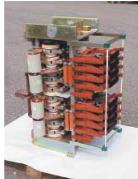
1 The basic building block of the Dynamic Voltage Restorer. Such modules can be combined to build different converter configurations and high-power DC-DC choppers.
