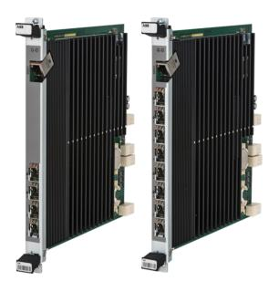
The encryption card SENC1 secures data transfer in critical infrastructures. It is used in mission-critical real-time applications for controlling and monitoring energy networks.
