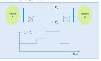
systems can be operated as merchant transmission facilities, similarly to merchant generators. The precise control of power flow through an HVDC Light system according to a contractual agreement simplifies the pricing of power transfers, billing, and preventing undesired flows **S**.
