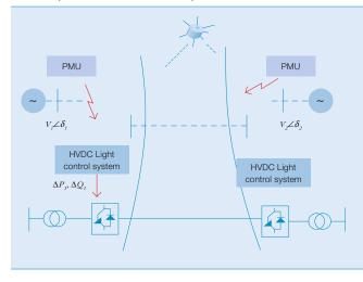
HVDC Light emulating an AC link in a post-disturbance situation. This mode is useful for mitigating possible overloading of adjacent AC lines.
