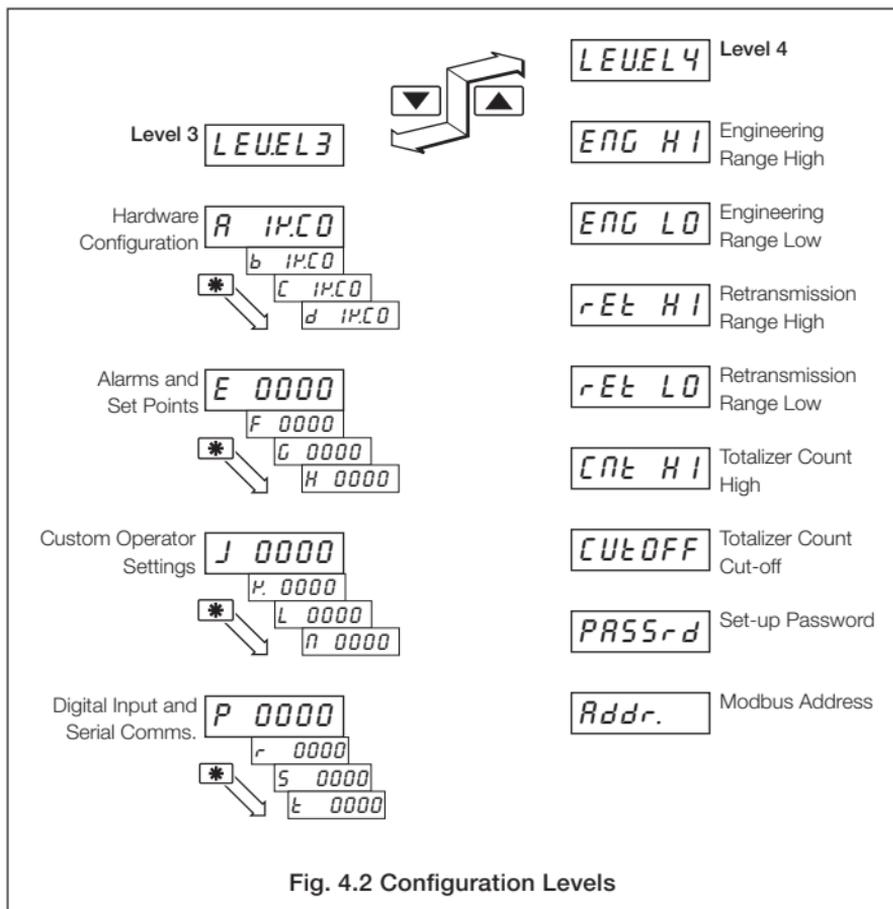
Fig. 4.2 Configuration Levels
