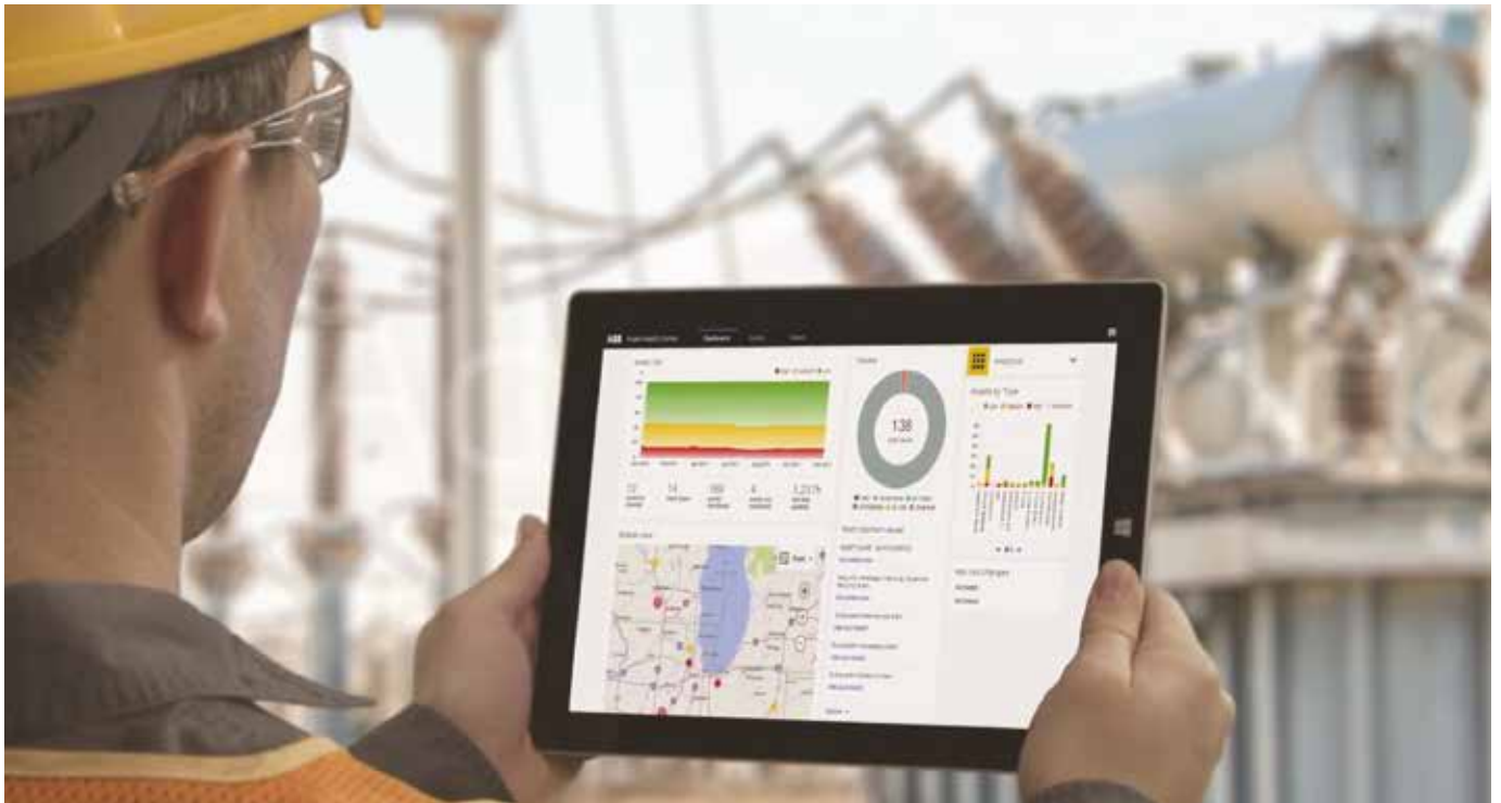
TXpert™ Asset Performance Management fleet analytic software ranking transformer risk of failure enabling maintenance to be prioritised
