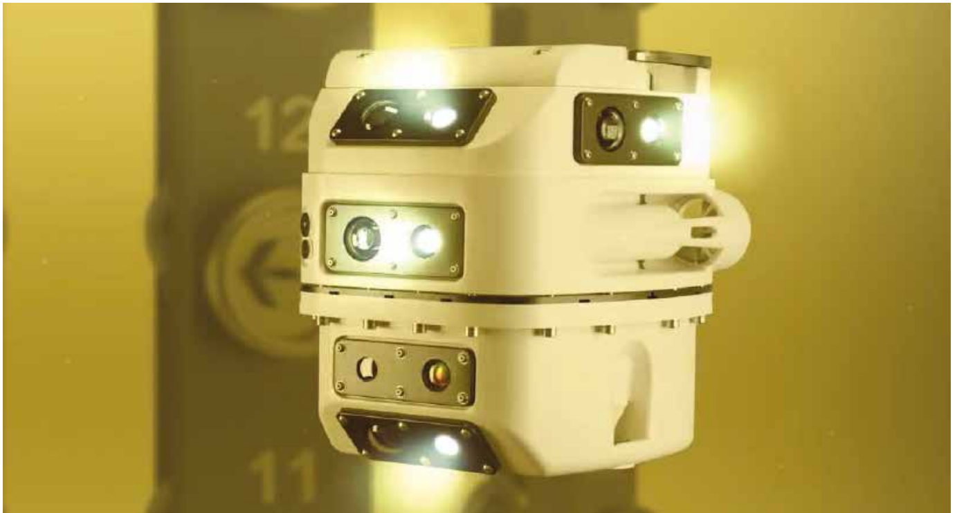
TXplore™ Inspection robot providing video fingerprint on internal transformer condition
