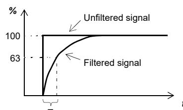
$O = I \times (1 - e^{-t/T})$ <p> <math>I</math> = filter input (step)<br/> <math>O</math> = filter output<br/> <math>t</math> = time<br/> <math>T</math> = filter time constant </p> <p><b>Note:</b> The signal is also filtered due to the signal interface hardware (approximately 0.25 ms time constant). This cannot be changed by any parameter.</p> | 0.100 s              |
