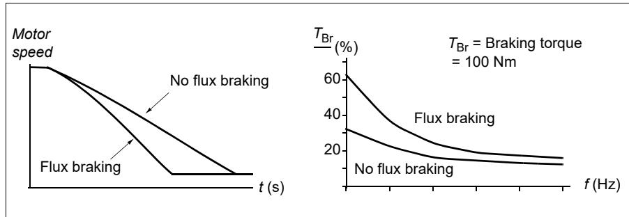
The drive monitors the motor status continuously, also during flux braking. Therefore, flux braking can be used both for stopping the motor and for changing the speed. The other benefits of flux braking are:
