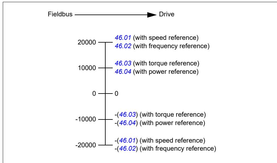
The scaled references are shown by parameters **03.09 EFB reference 1** and **03.10 EFB reference 2**.
