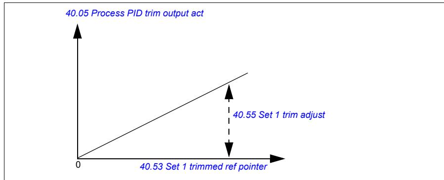
**Note:** In the above graph, it is assumed that the PID output is limited or stable at 100. This is for understanding purpose only. In real case scenario, PID output can vary based on the setpoint and actual.
