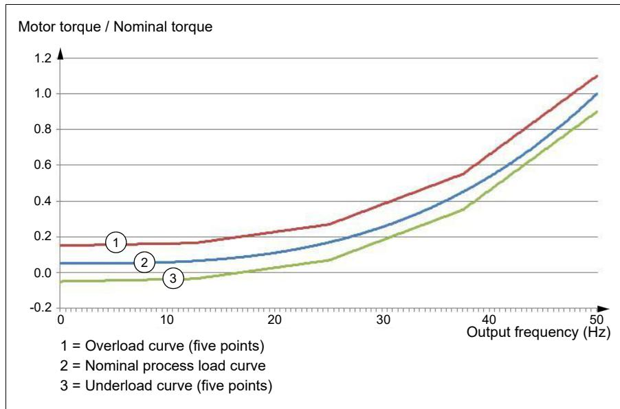
An overload warning and/or fault can be set to occur if the monitored signal stays continuously over the overload curve for a defined time. An underload warning and/or fault can be set to occur if the monitored signal stays continuously under the underload for a defined time.
