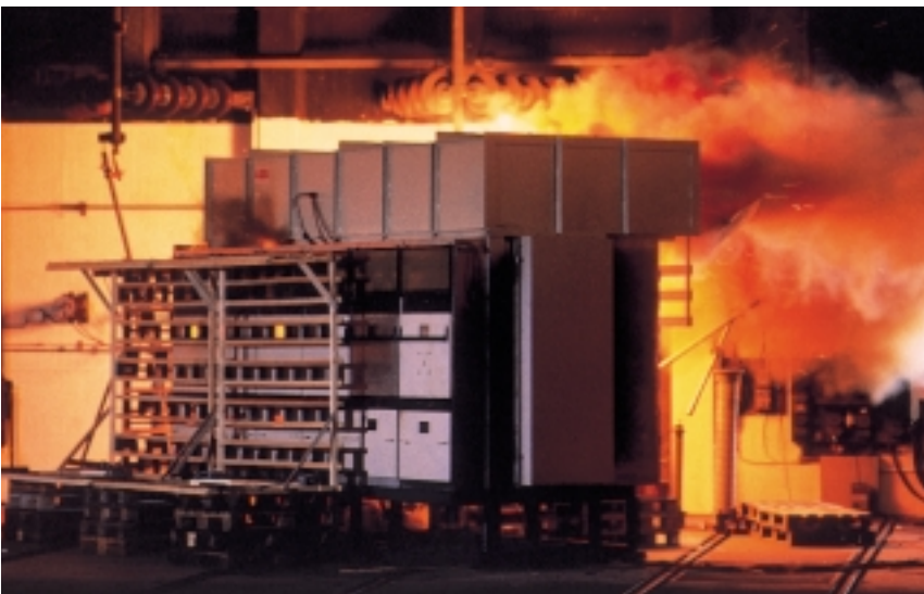
Short-circuit test being carried out in the high power laboratory in Ludvika
