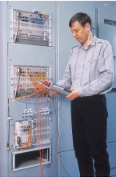
Analogue/digital converter for the collection of measurement data 5
