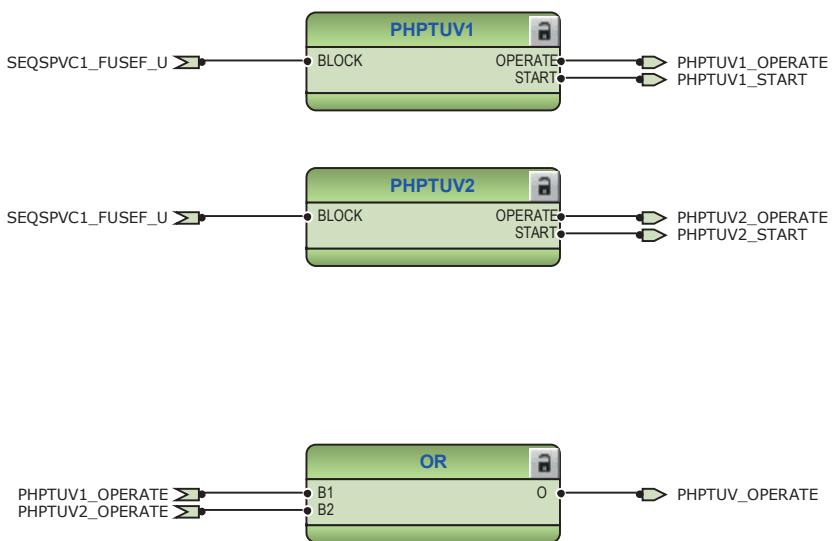
Figure 65: Undervoltage protection function
