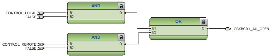
Figure 41: External opening command for circuit breaker
