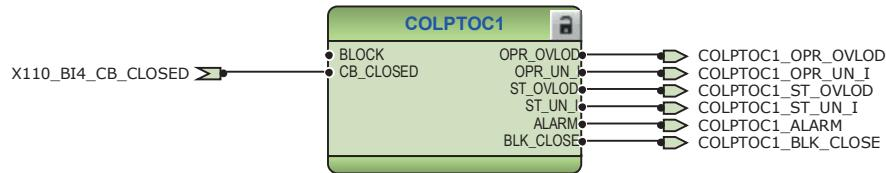
Figure 61: Capacitor bank overload protection function
