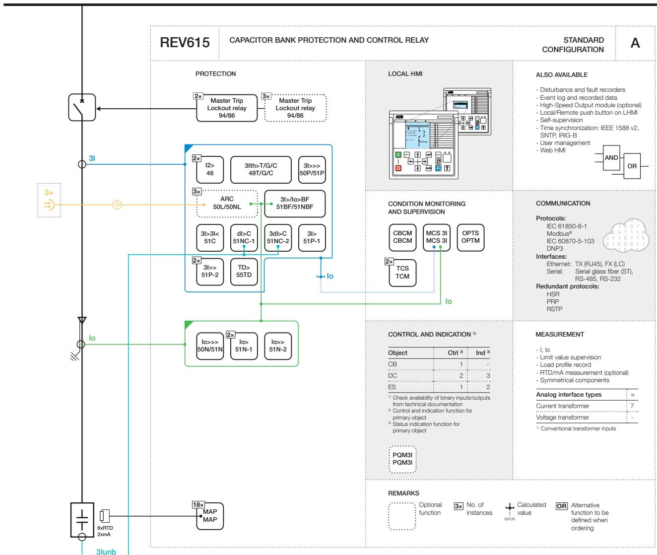
Figure 13: Functionality overview for standard configuration A
