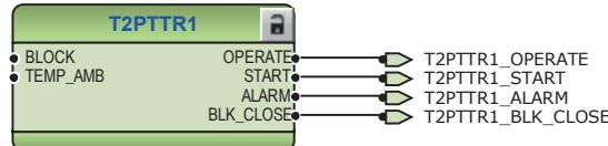
*Figure 17: Thermal overcurrent protection function*
