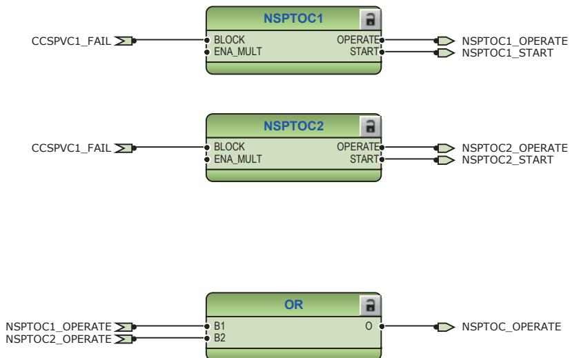
Figure 56: Negative-sequence overcurrent protection function
