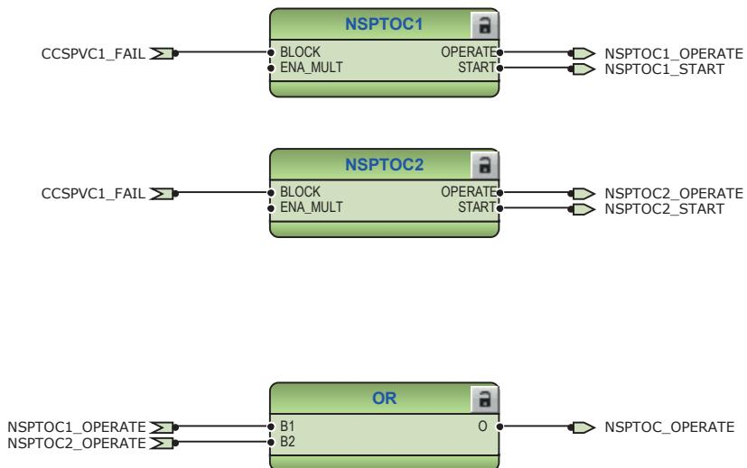
Figure 15: Negative-sequence overcurrent protection function
