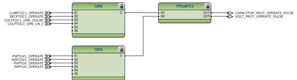
Figure 104: Timer logic for capacitor protection and voltage protection operate pulse
