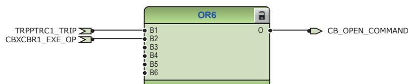
*Figure 37: Circuit breaker control logic: Signals for opening coil of circuit breaker*
