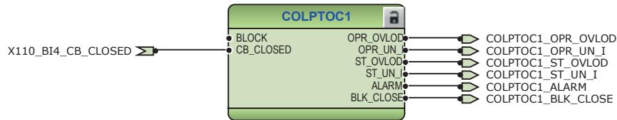
*Figure 20: Capacitor bank overload protection function*
