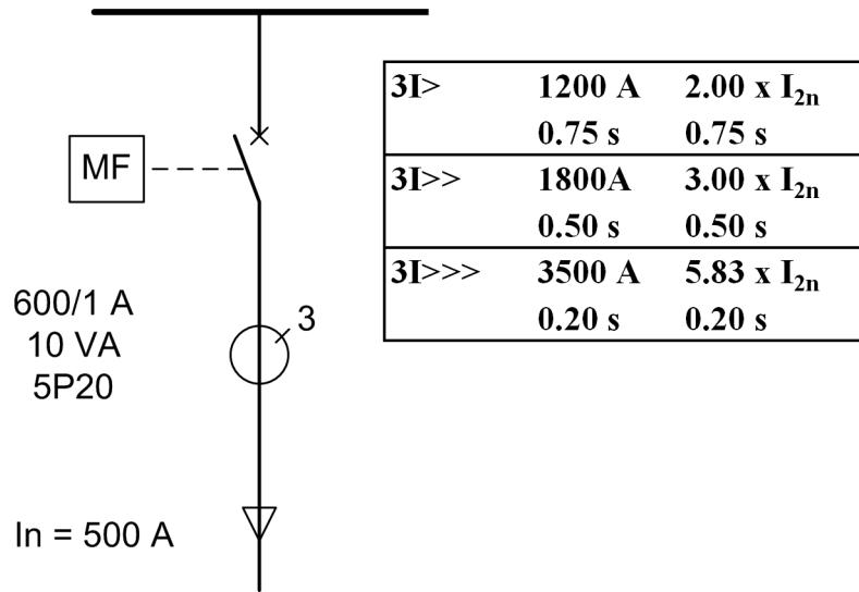
Figure 106: Example of three-stage overcurrent protection
