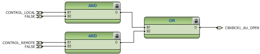
Figure 88: External opening command for circuit breaker
