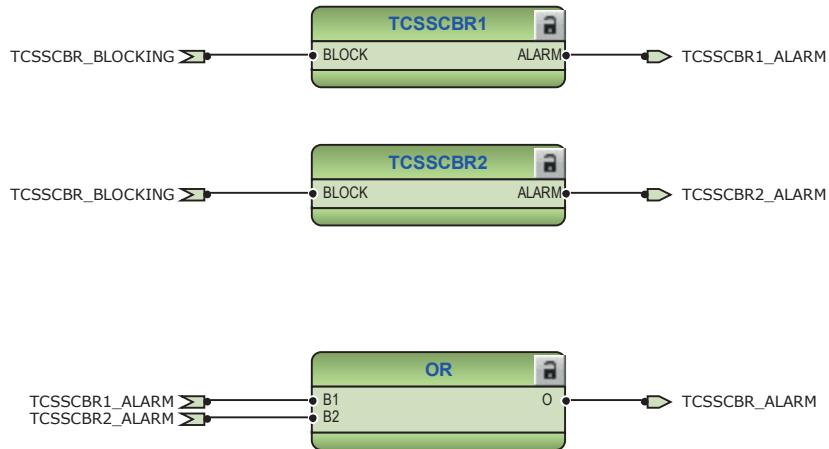
Figure 31: Trip circuit supervision function
