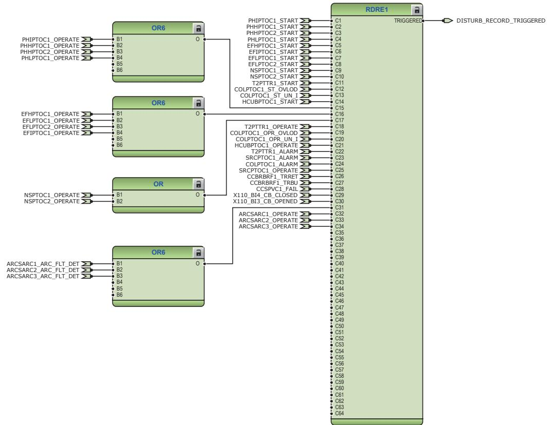
Figure 26: Disturbance recorder
