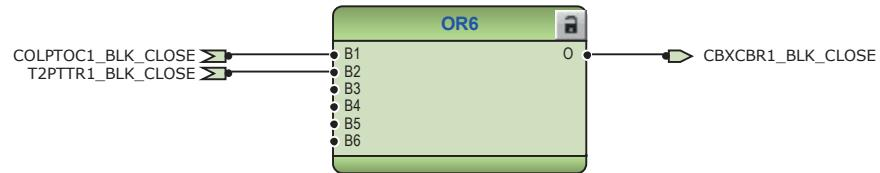
Figure 86: Circuit breaker close blocking logic
