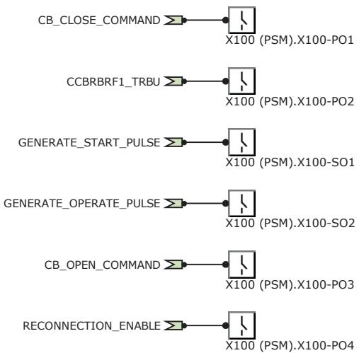
*Figure 49: Binary outputs - X100 terminal block*
