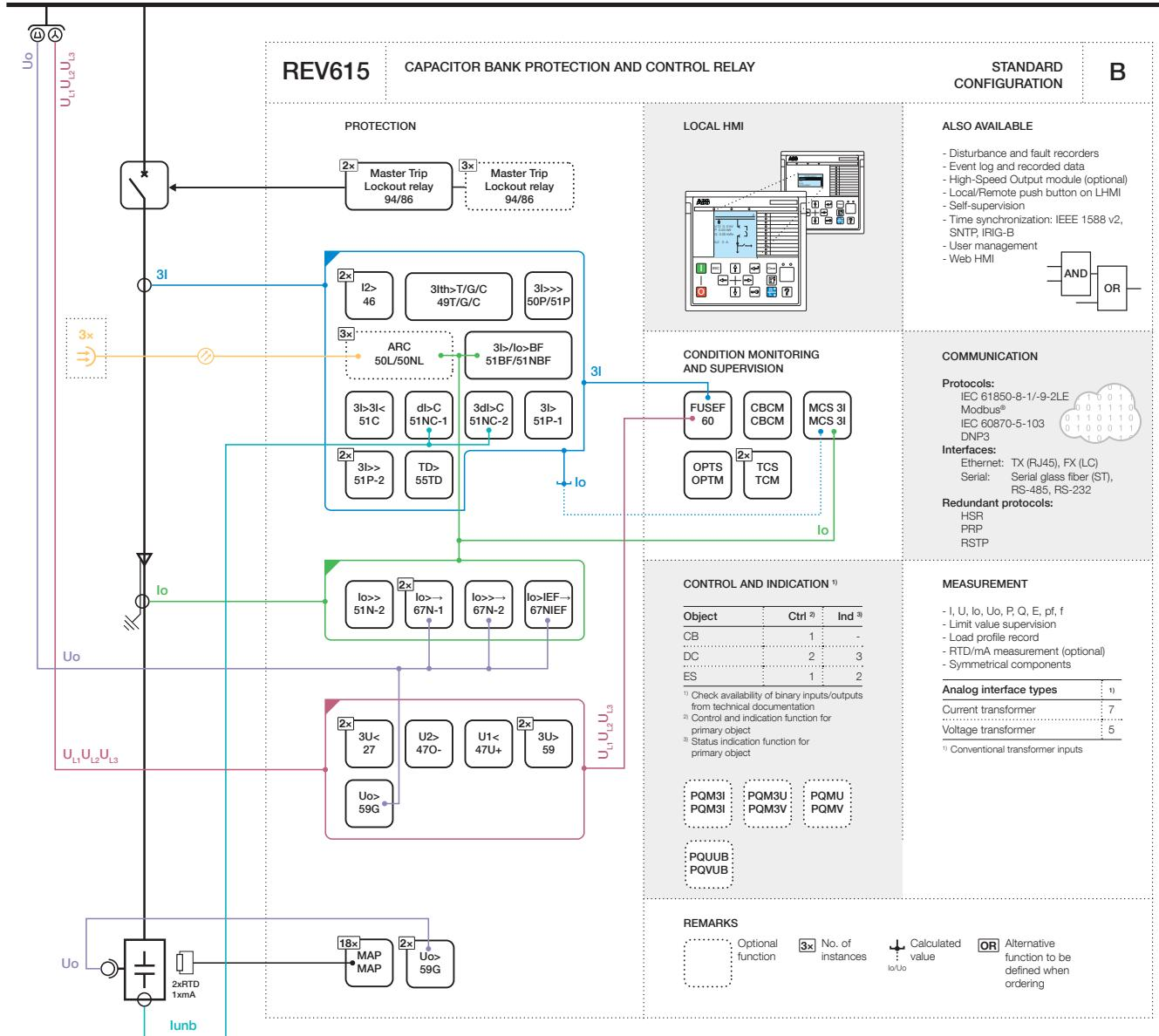
Figure 54: Functionality overview for standard configuration B
