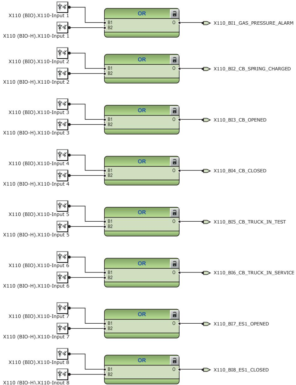
Figure 47: Default binary inputs - X110 terminal block
