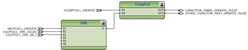
*Figure 52: Timer logic for capacitor unbalance and other capacitor protection operate pulse*
