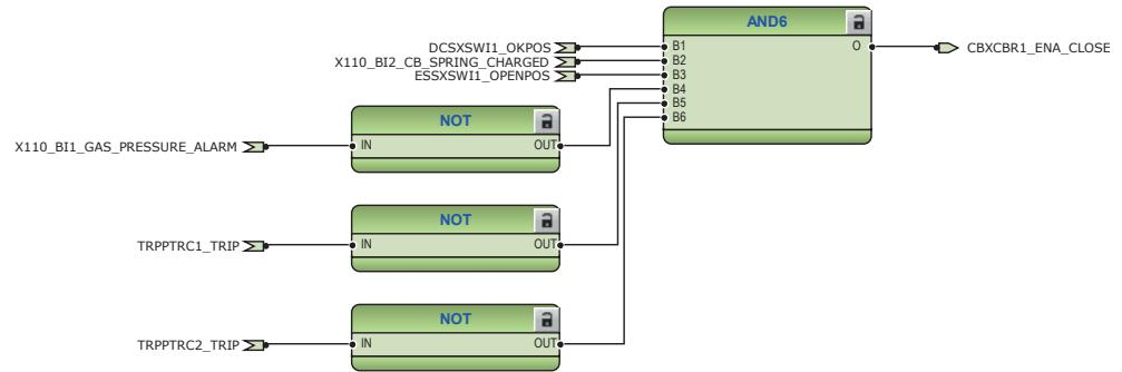
Figure 38: Circuit breaker close enable logic
