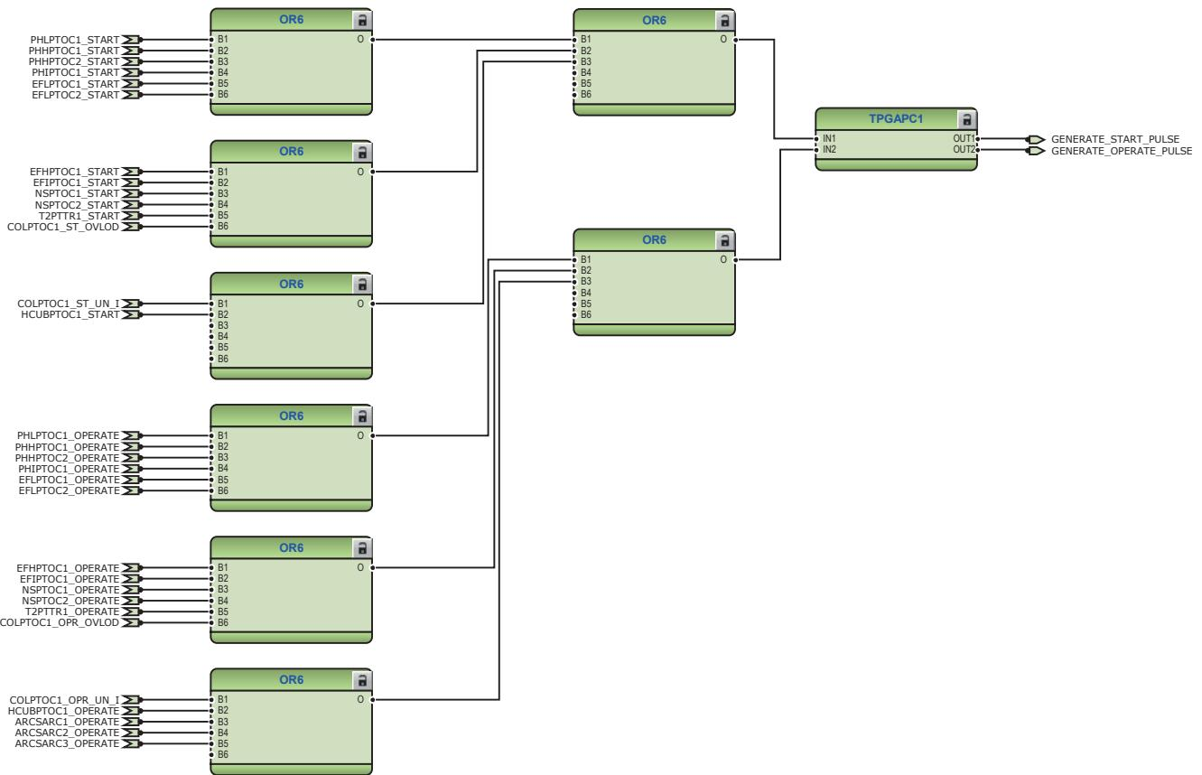
*Figure 23: General start and operate signals*
