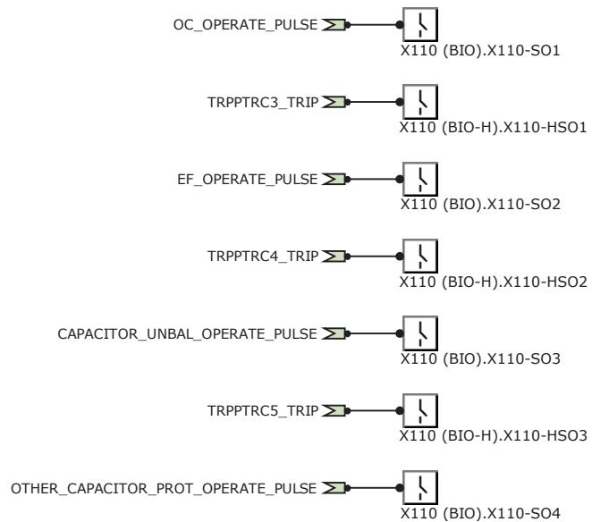
*Figure 48: Binary outputs - X110 terminal block*
