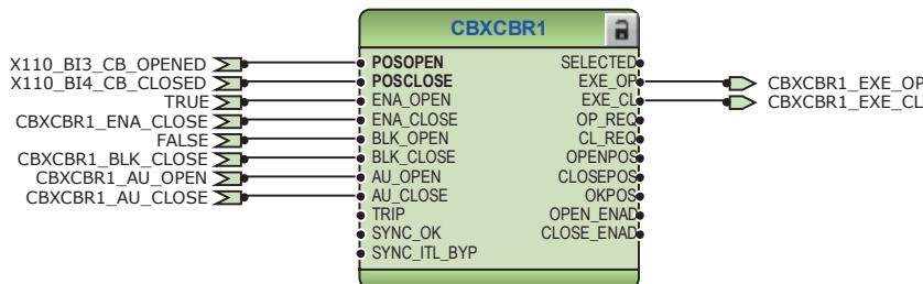
*Figure 82: Circuit breaker control logic: Circuit breaker 1*
