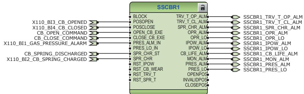
Figure 28: Circuit-breaker condition monitoring function
