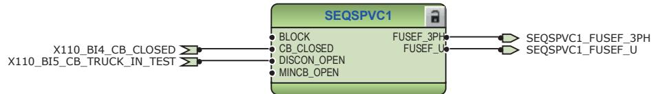
*Figure 74: Fuse failure supervision function*
