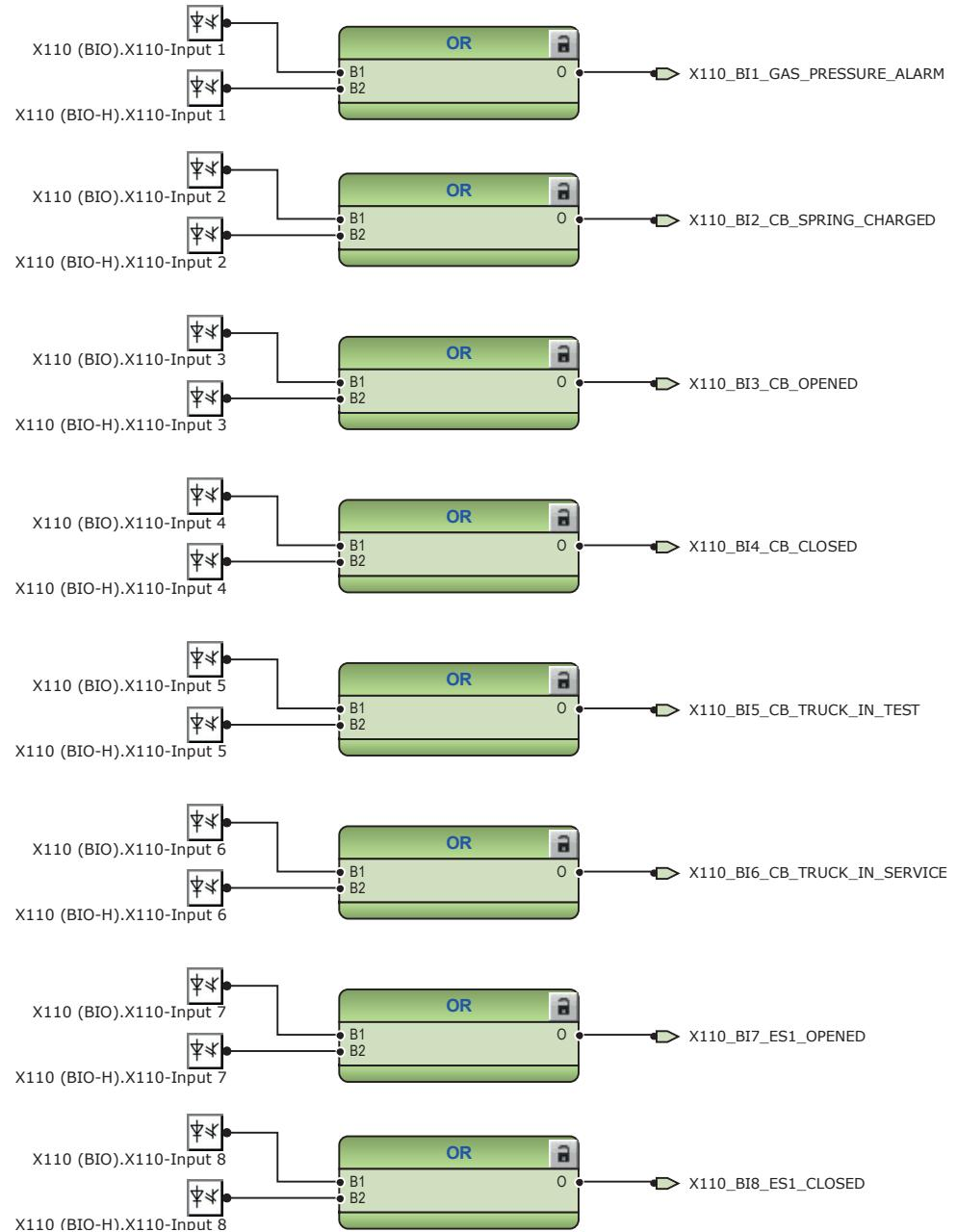
Figure 99: Default binary inputs - X110 terminal block
