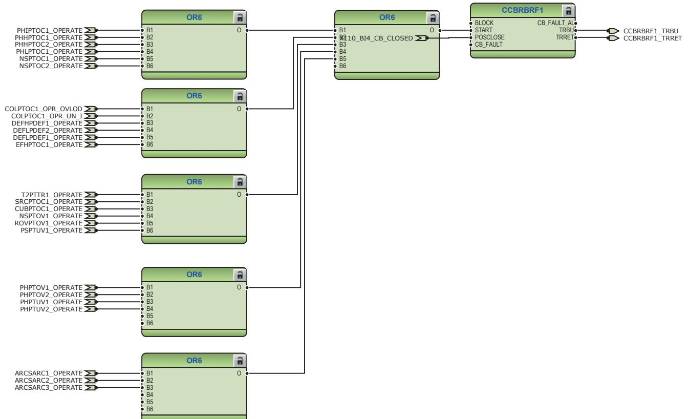
*Figure 59: Circuit breaker failure protection function*
