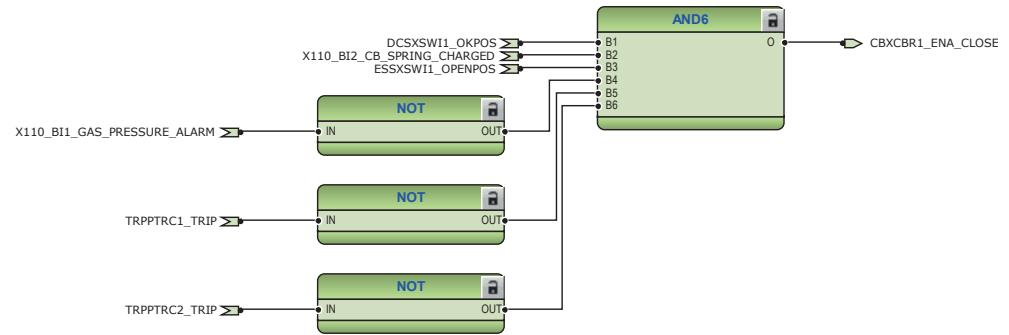
Figure 85: Circuit breaker close enable logic
