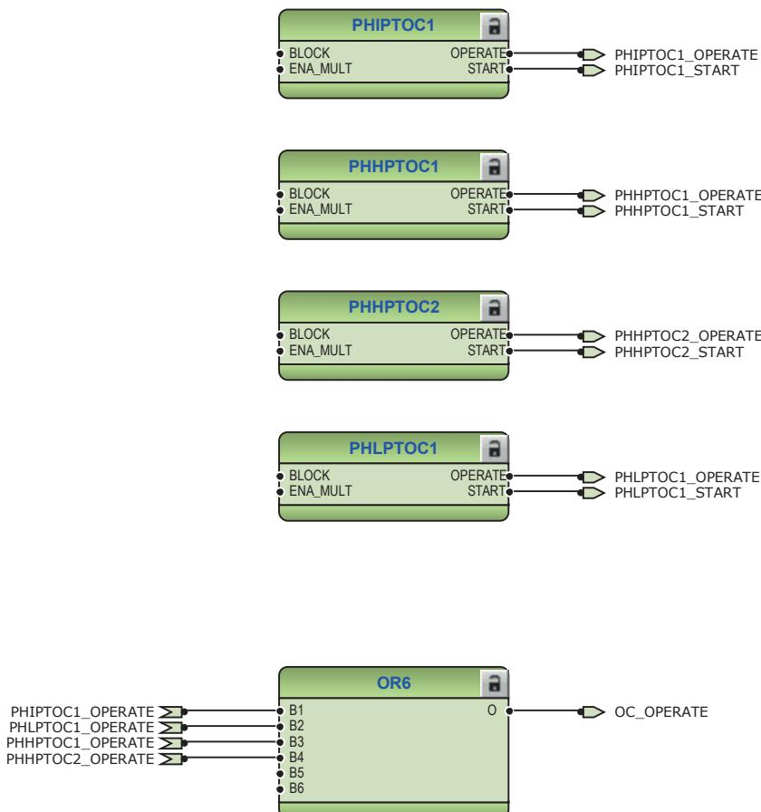
Figure 14: Overcurrent protection functions
