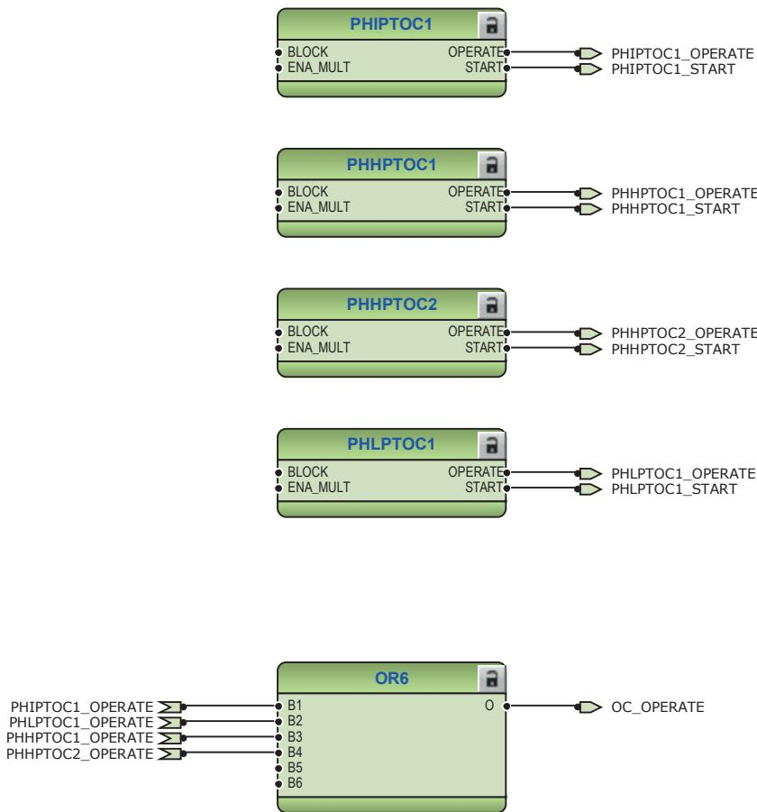
Figure 55: Overcurrent protection functions
