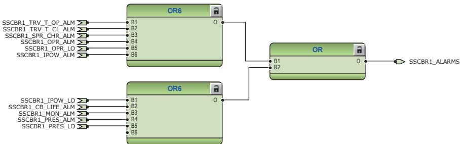
Figure 29: Logic for circuit breaker monitoring alarm
