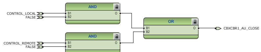
Figure 40: External closing command for circuit breaker
