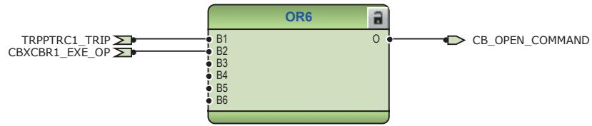
Figure 84: Circuit breaker control logic: Signals for opening coil of circuit breaker
