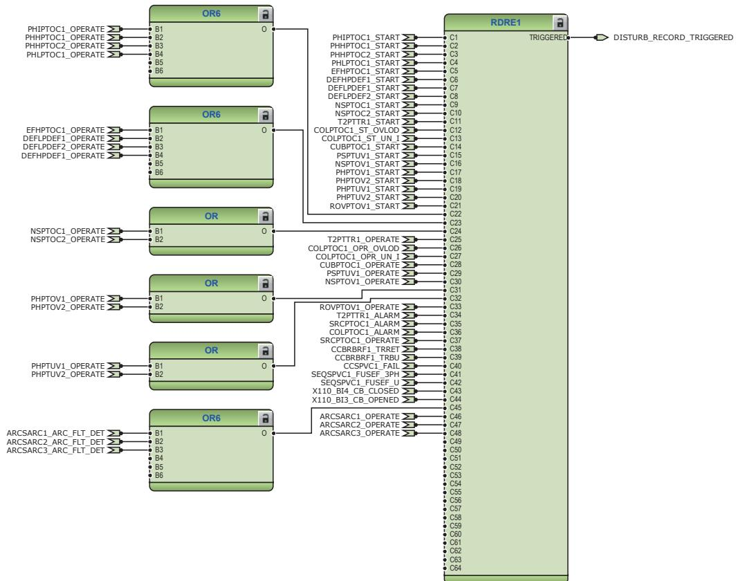
Figure 72: Disturbance recorder
