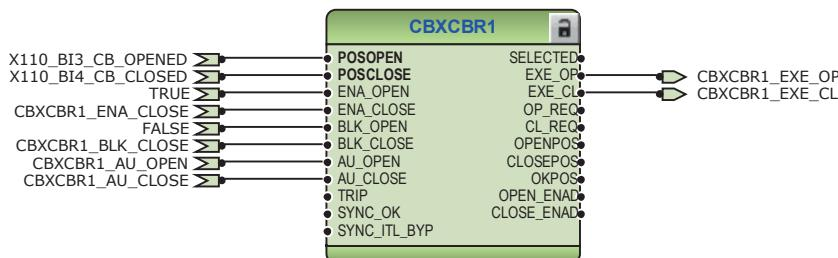
*Figure 35: Circuit breaker control logic: Circuit breaker 1*
