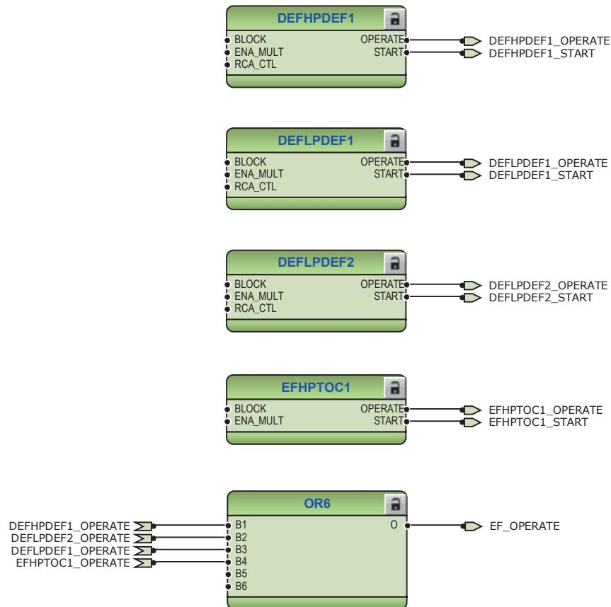
Figure 57: Earth-fault protection functions
