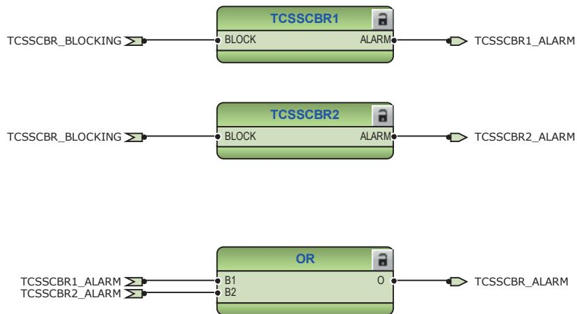
Figure 78: Trip circuit supervision function
