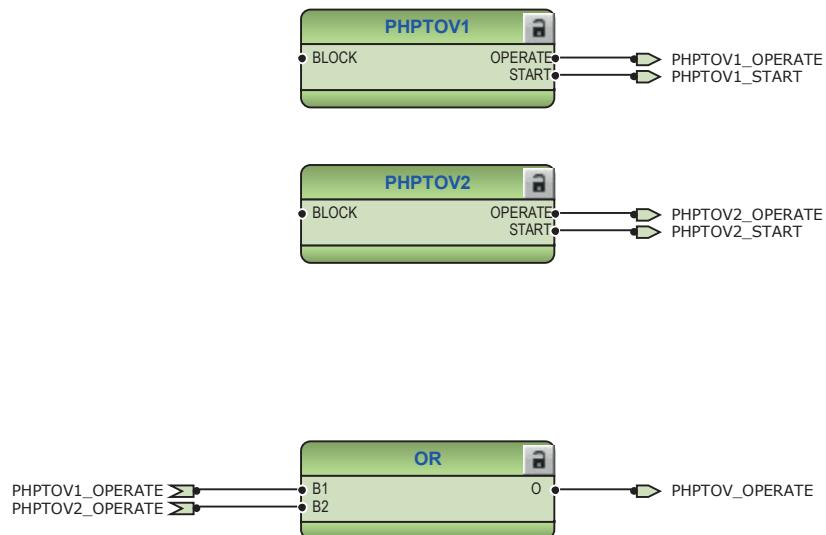
Figure 64: Overvoltage protection function
