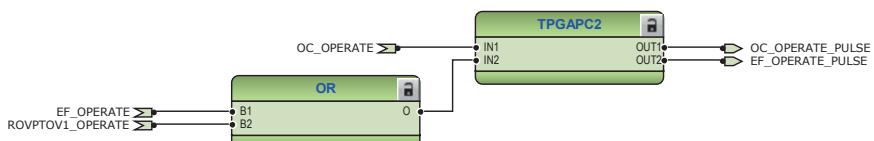
Figure 103: Timer logic for overcurrent and earth-fault operate pulse
