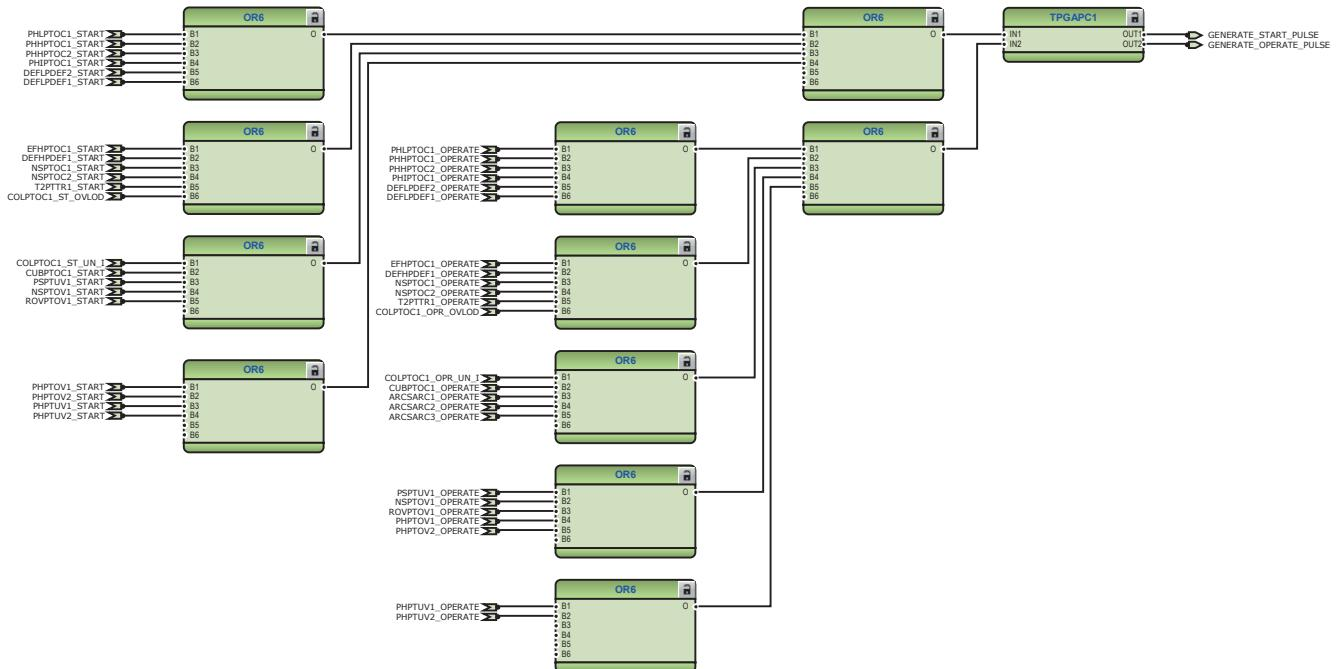
*Figure 69: General start and operate signals*
