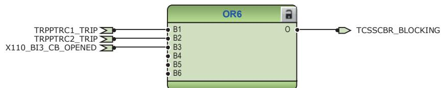
Figure 79: Logic for blocking trip circuit supervision function
