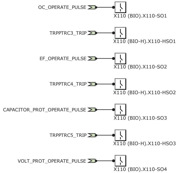
*Figure 100: Binary outputs - X110 terminal block*
