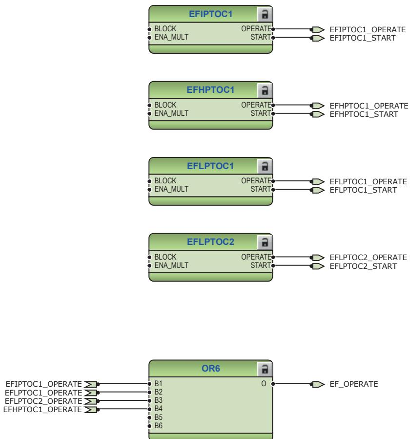
Figure 16: Earth-fault protection functions
