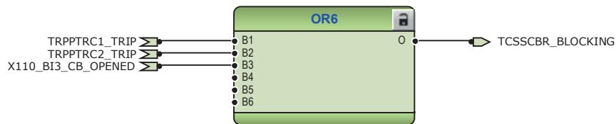
Figure 32: Logic for blocking trip logic circuit supervision
