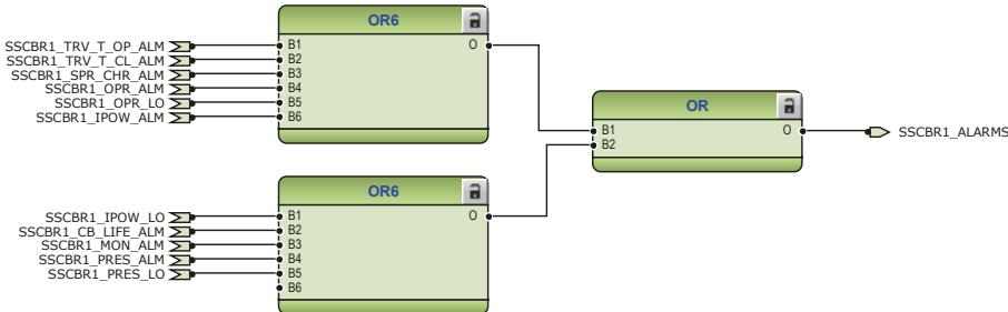
*Figure 76: Logic for circuit breaker monitoring alarm*
