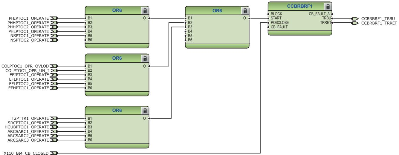
*Figure 18: Circuit breaker failure protection function*
