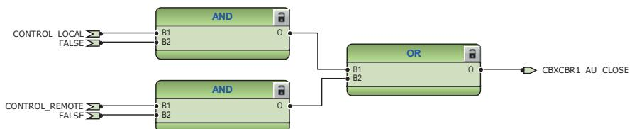
Figure 87: External closing command for circuit breaker
