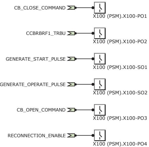
*Figure 101: Binary outputs - X100 terminal block*
